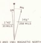
UTM GRID AND 1961 MAGNETIC NORTH DECLINATION AT CENTER OF SHEET
