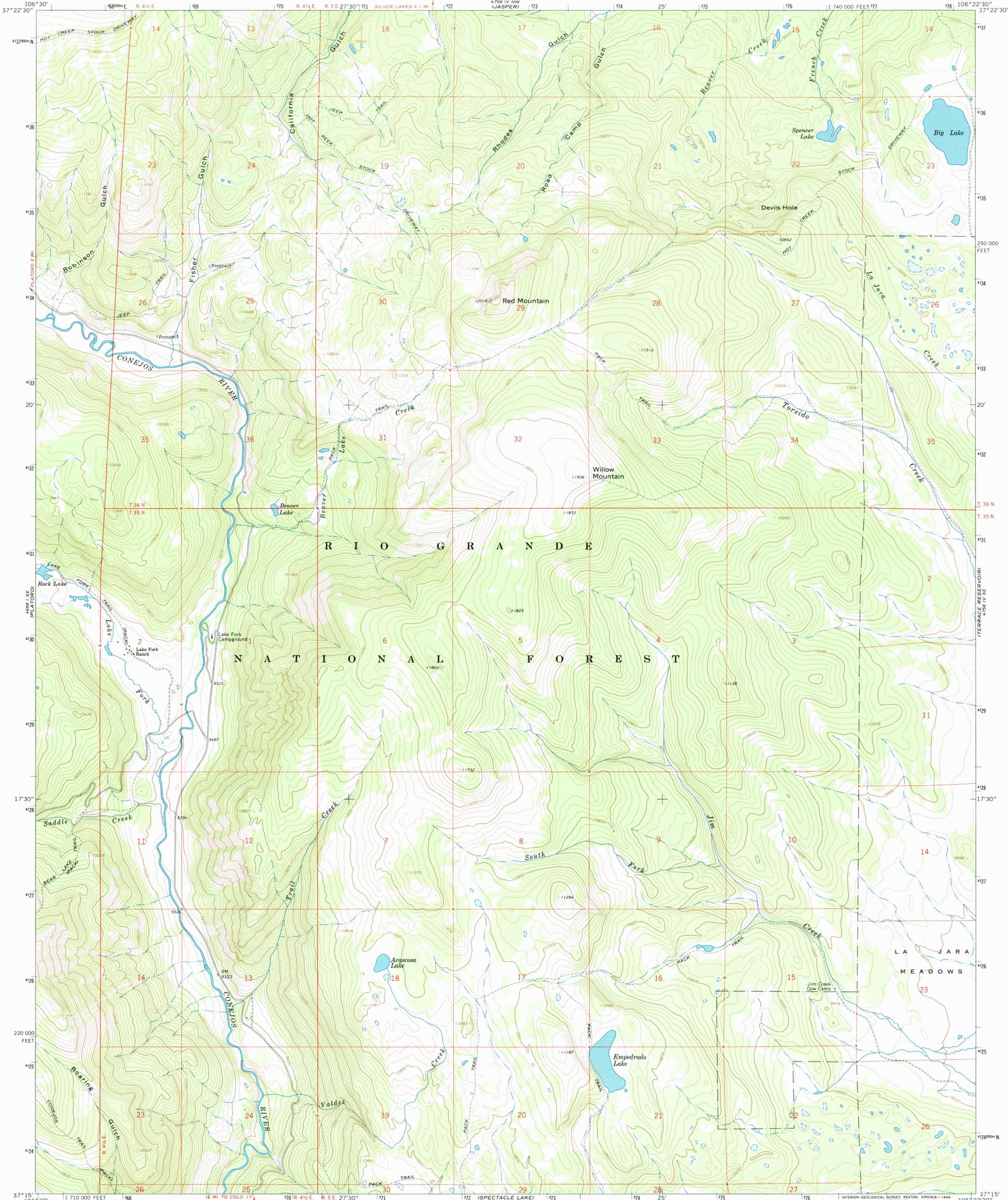
Mapped by the U. S. Forest Service Edited and published by the Geological Survey Control by USGS, USC&GS, and U. S. Forest Service Topography by photogrammetric methods from aerial photographs taken 1960-1961. Field checked USGS 1967 Polyconic projection. 1927 North American datum 10,000-foot grid based on Colorado coordinate system, south zone 1000-meter Universal Transverse Mercator grid ticks, zone 13, shown in blue Certain land lines are omitted because of insufficient data
