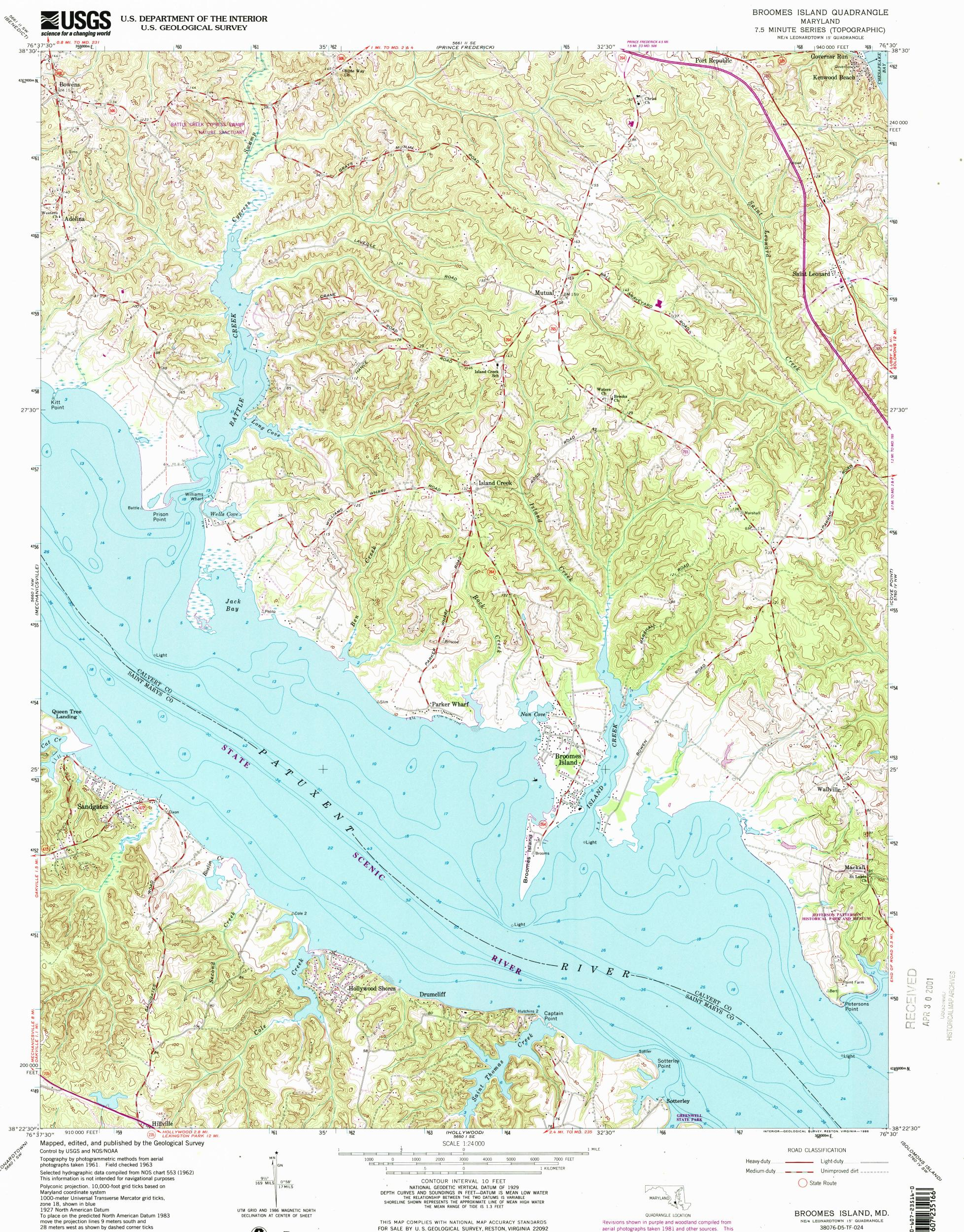
Polyconic projection. 10,000-foot grid ticks based on Maryland coordinate system 1000-meter Universal Transverse Mercator grid ticks, zone 18, shown in blue 1927 North American Datum To place on the predicted North American Datum 1983 move the projection lines 9 meters south and 28 meters west as shown by dashed corner ticks
