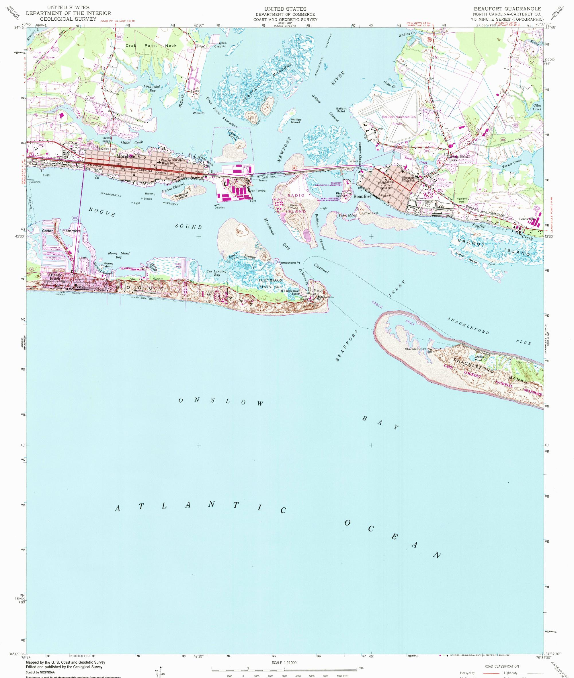
Planimetry in part by photogrammetric methods from aerial photographs taken 1946. Topography by planetable surveys 1947
