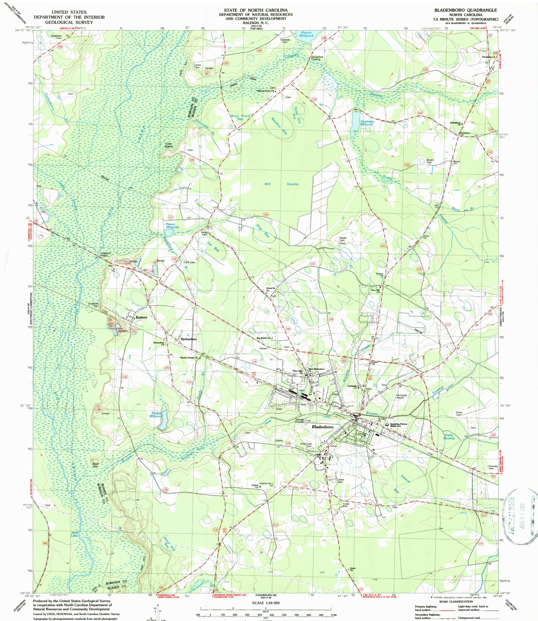
taken 1979. Field checked 1981. Map edited 1986 Projection and 10,000-foot grid ticks: North Carolina coordinate system, (Lambert conformal conic) 1000-meter Universal Transverse Mercator grid, zone 17 1927 North American Datum To place on the predicted North American Datum 1983, move the projection lines 13 meters south and 23 meters west as shown by dashed corner ticks
