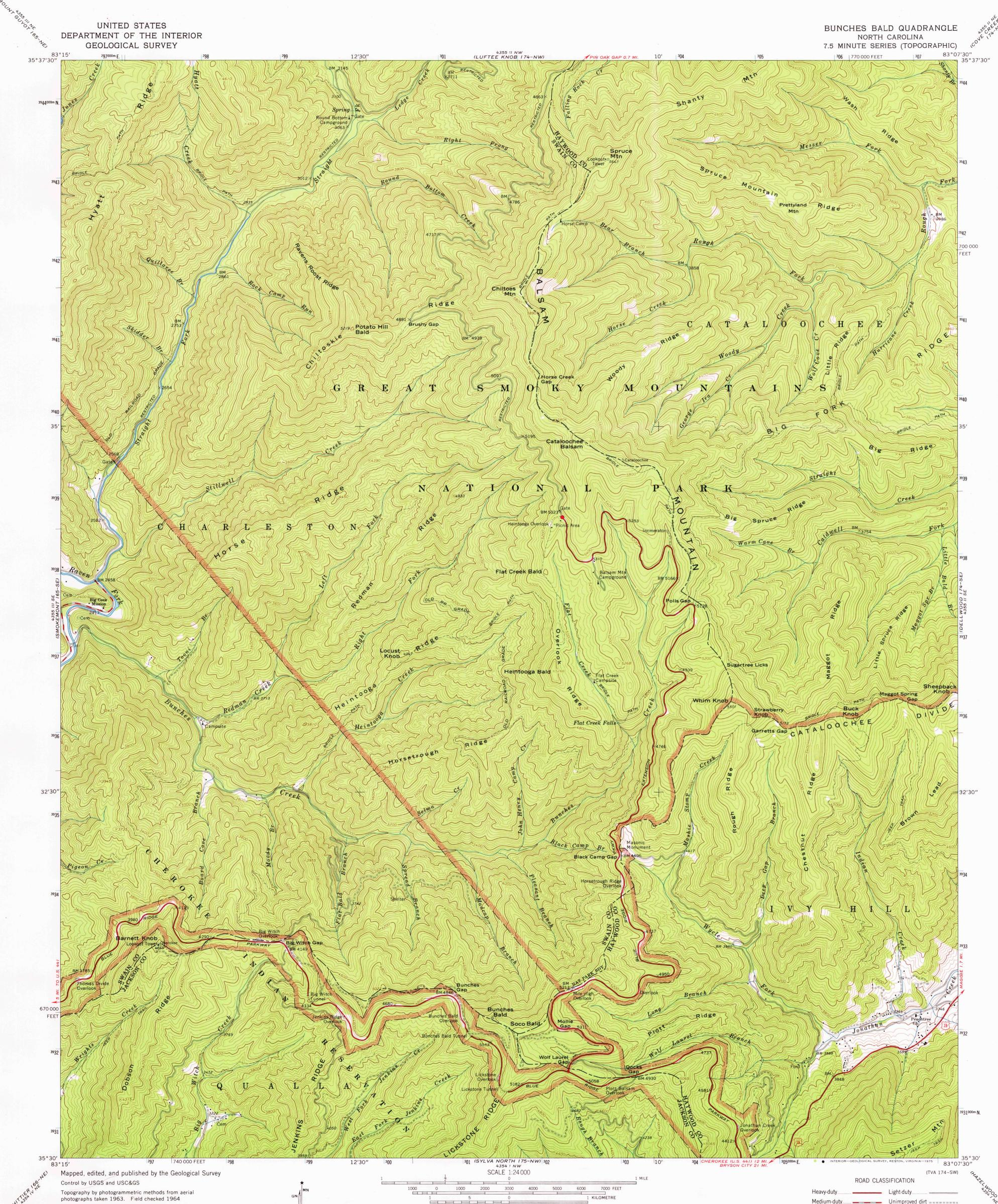
Polyconic projection. 1927 North American datum 10,000-foot grid based on North Carolina coordinate system 1000-metre Universal Transverse Mercator grid ticks, zone 17, shown in blue
