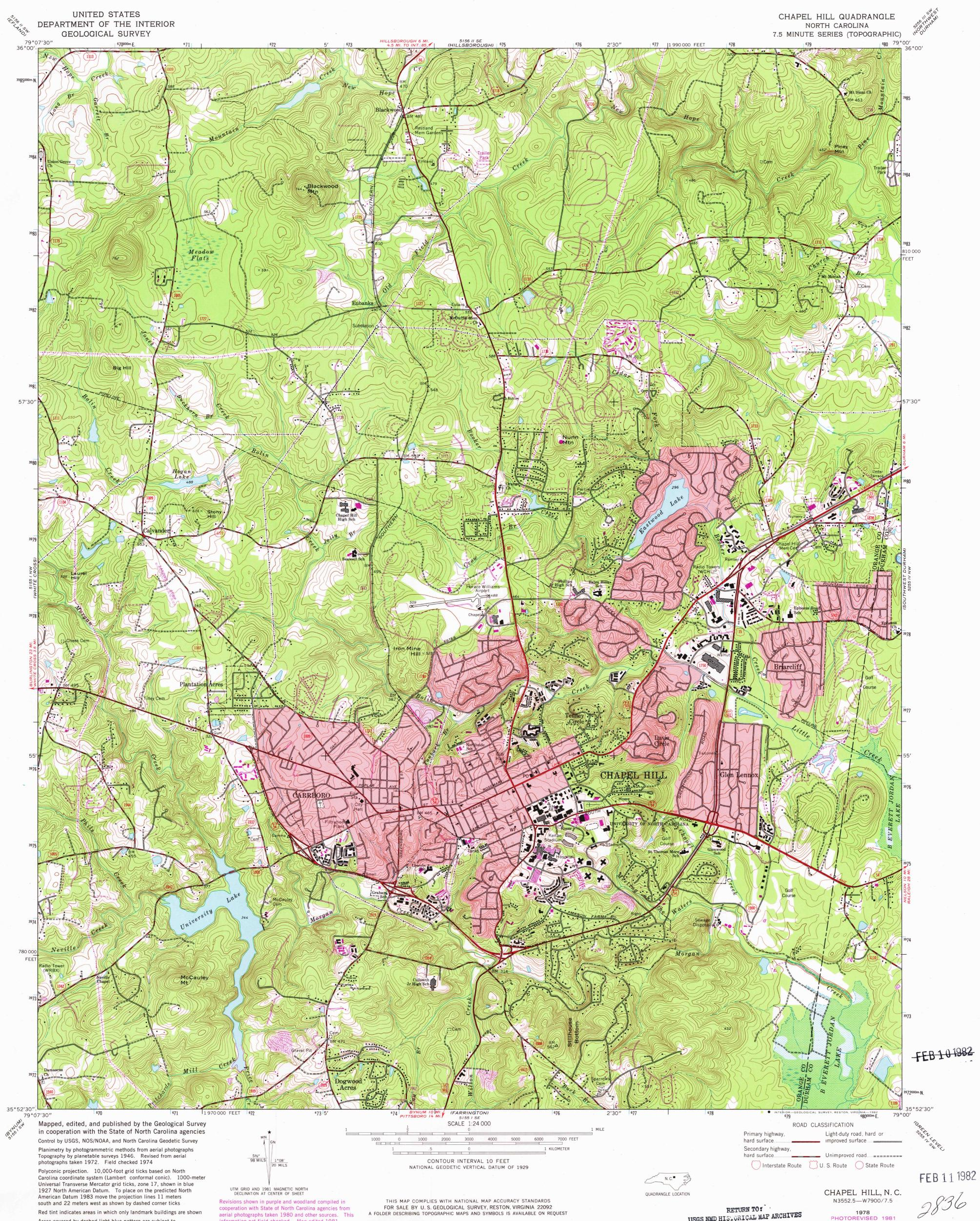
Polyconic projection. 10,000-foot grid ticks based on North Carolina coordinate system (Lambert conformal conic). 1000-meter Universal Transverse Mercator grid ticks, zone 17, shown in blue 1927 North American Datum. To place on the predicted North American Datum 1983 move the projection lines 11 meters south and 22 meters west as shown by dashed corner ticks
