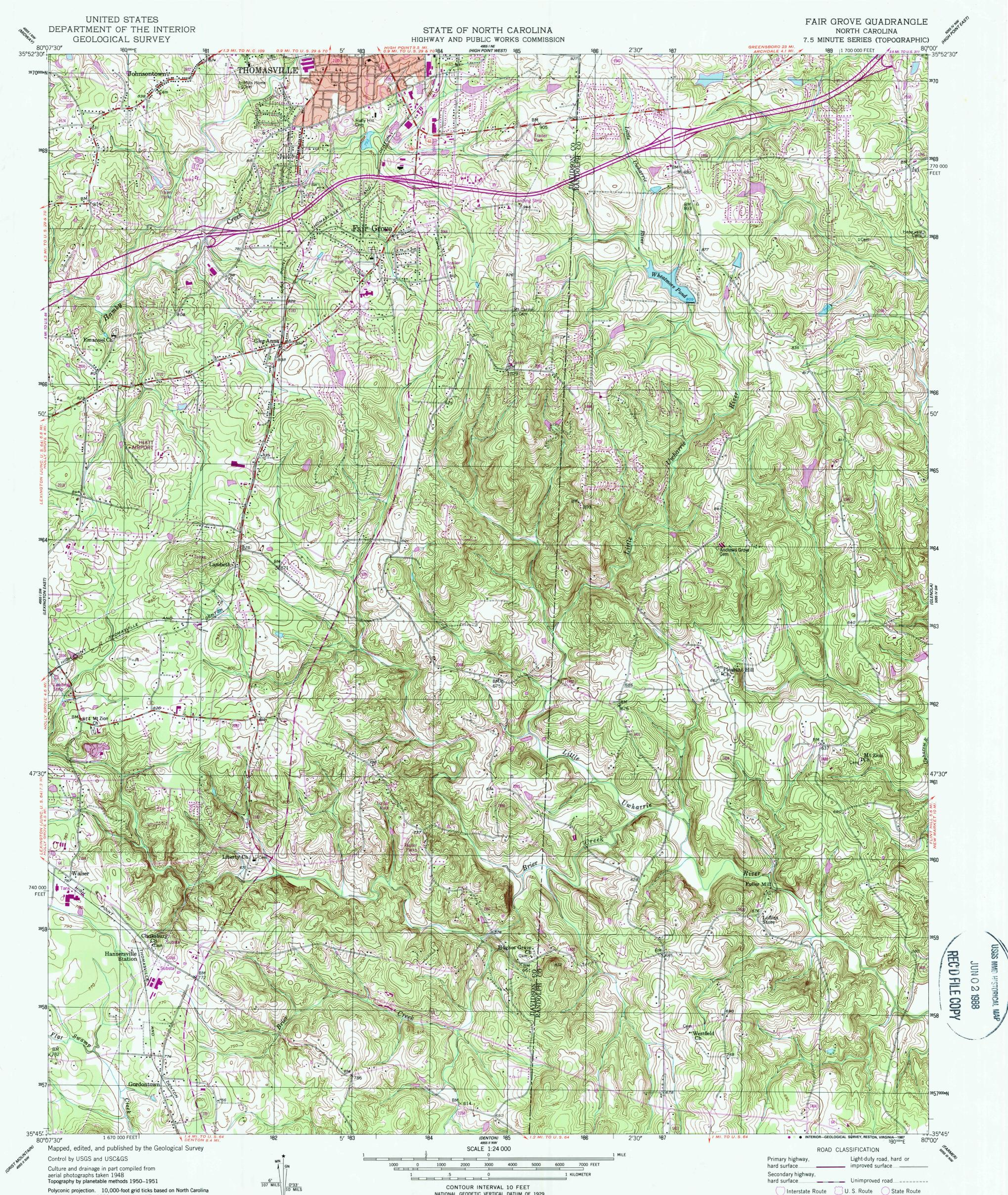
Polyconic projection. 10,000-foot grid ticks based on North Carolina coordinate system. 1000-meter Universal Transverse Mercator grid ticks, zone 17. 1927 North American Datum. To place on the predicted North American Datum 1983 move the projection lines 10 meters south and 19 meters west as shown by dashed corner ticks Red tint indicates areas in whick only landmark buildings are shown
