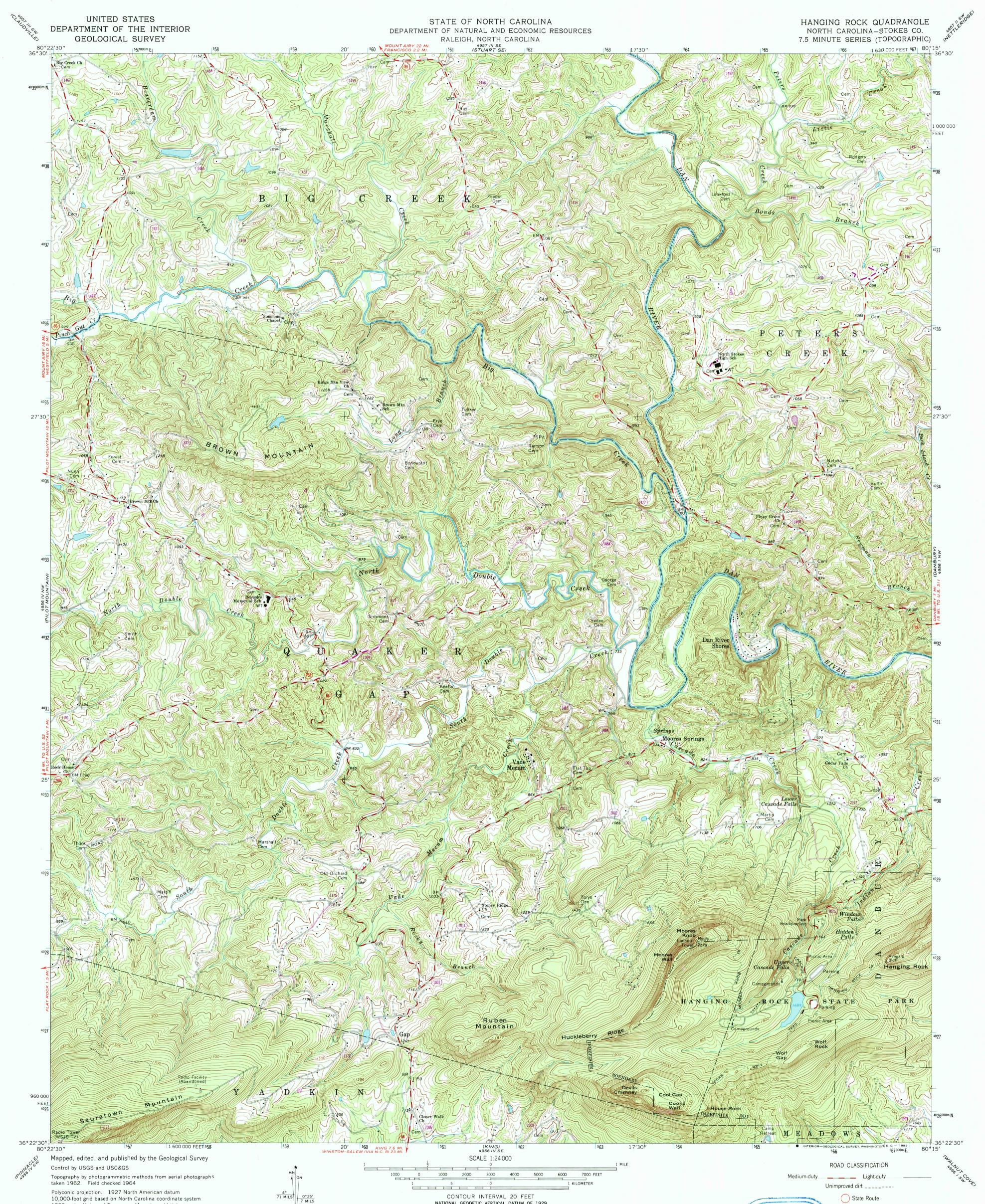
Polyconic projection. 1927 North American datum 10,000-foot grid based on North Carolina coordinate system 1000-meter Universal Transverse Mercator grid ticks, zone 17, shown in blue The difference between 1927 North American Datum and North American Datum of 1983 (NAD 83) for 7.5-minute intersections is given in USGS Bulletin 1875. The NAD 83 is shown by dashed corner ticks Revisions shown in purple compiled from aerial photographs taken 1971. This information not field checked
