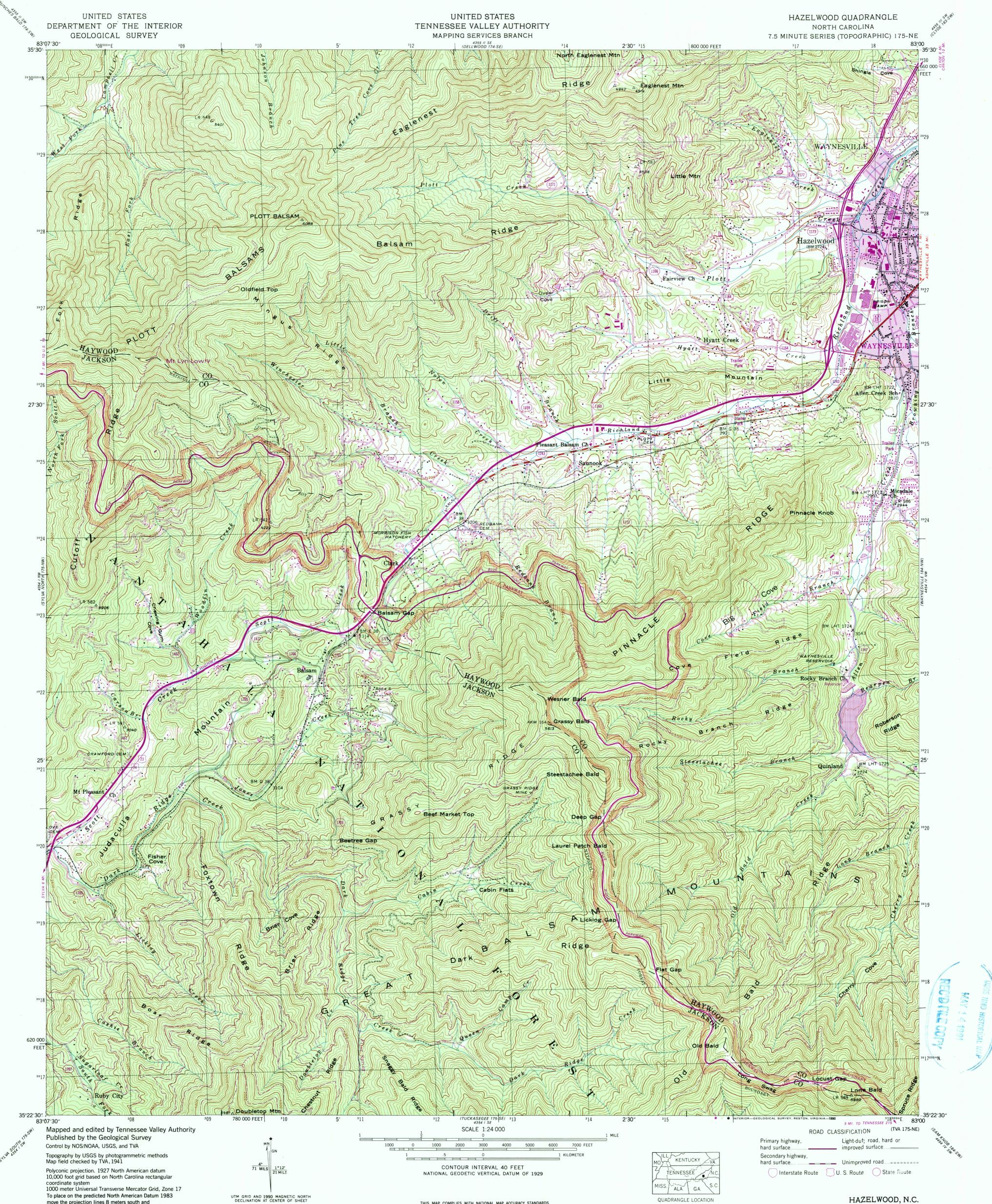
To place on the predicted North American Datum 1983 move the projection lines 8 meters south and 11 meters west as shown by dashed corner ticks
