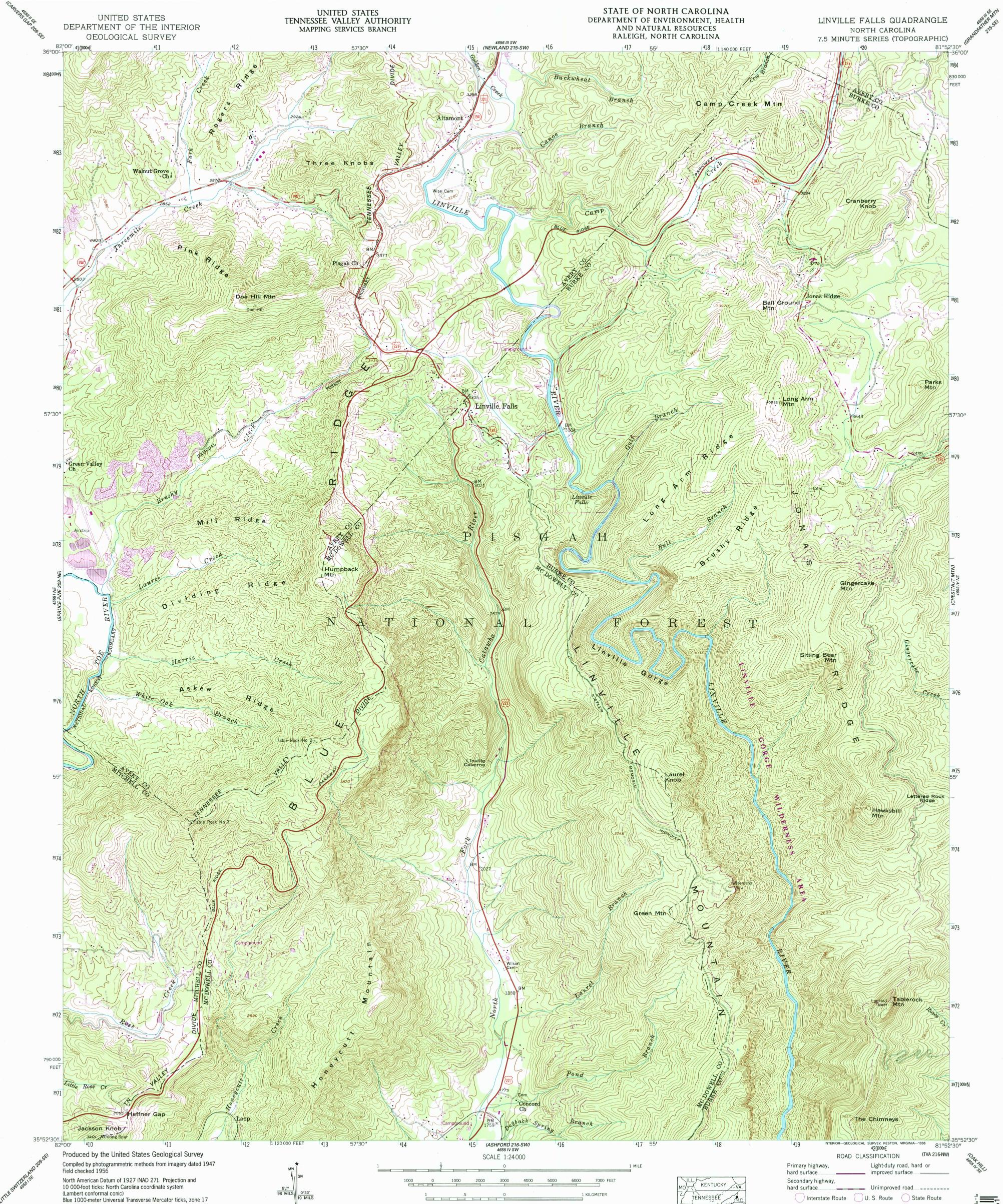
North American Datum of 1983 (NAD 83) is shown by dashed corner ticks. The values of the shift between NAD 27 and NAD 83 for 7.5-minute intersections are obtainable from National Geodetic Survey NADCON software
