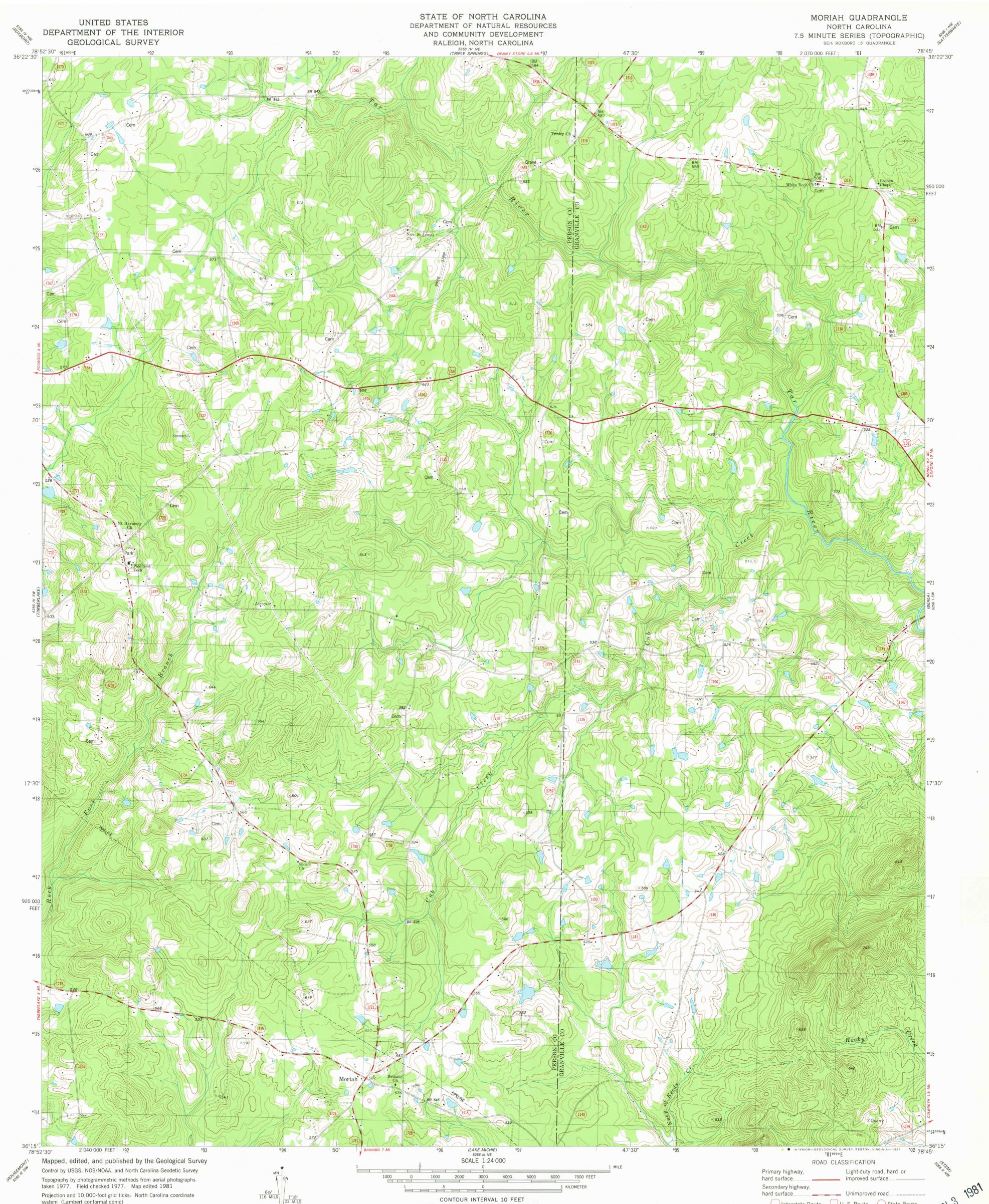
system (Lambert conformal conic) 1000-meter Universal Transverse Mercator grid, zone 17 1927 North American Datum To place on the predicted North American Datum 1983 move the projection lines 12 meters south and 23 meters west as shown by dashed corner ticks
