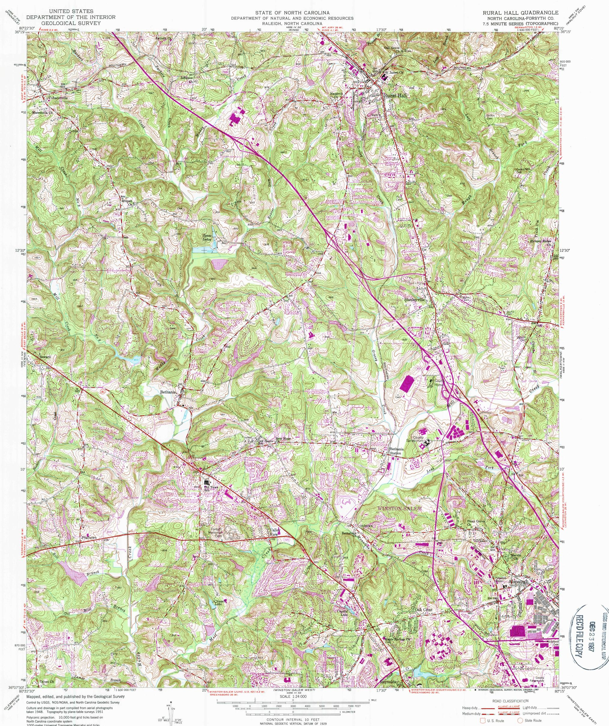
Polyconic projection. 10,000-foot grid ticks based on North Carolina coordinate system 1000-meter Universal Transverse Mercator grid ticks, zone 17, shown in blue 1927 North American Datum To place on the predicted North American Datum 1983 move the projection lines 10 meters south and 18 meters west as shown by dashed corner ticks
