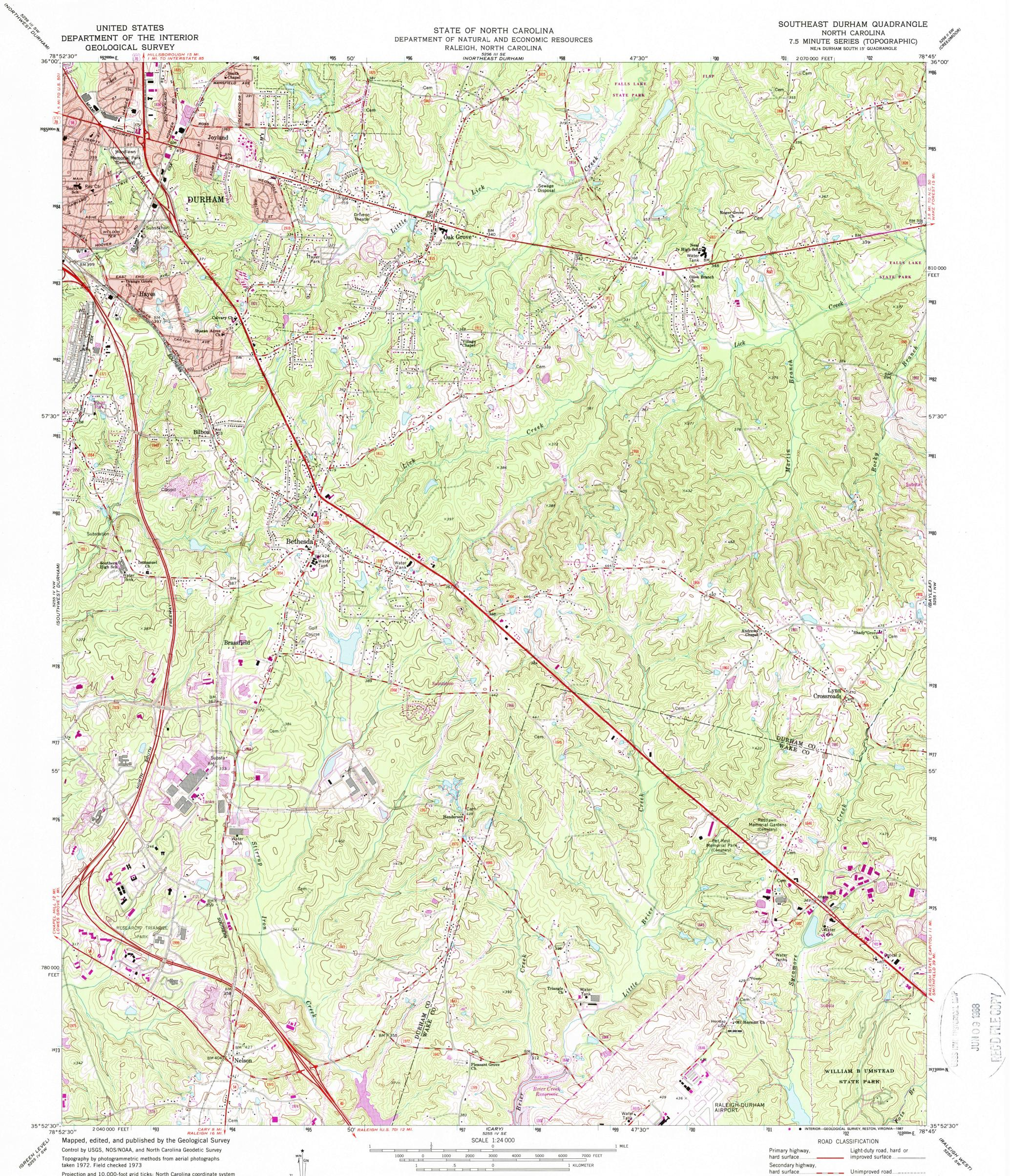
Projection and 10,000-foot grid ticks: North Carolina coordinate system (Lambert conformal conic). 1000-meter Universal Transverse Mercator grid ticks, zone 17, shown in blue. 1927 North American Datum To place on the predicted North American Datum 1983 move the projection lines 11 meters south and 23 meters west as shown by dashed corner ticks
