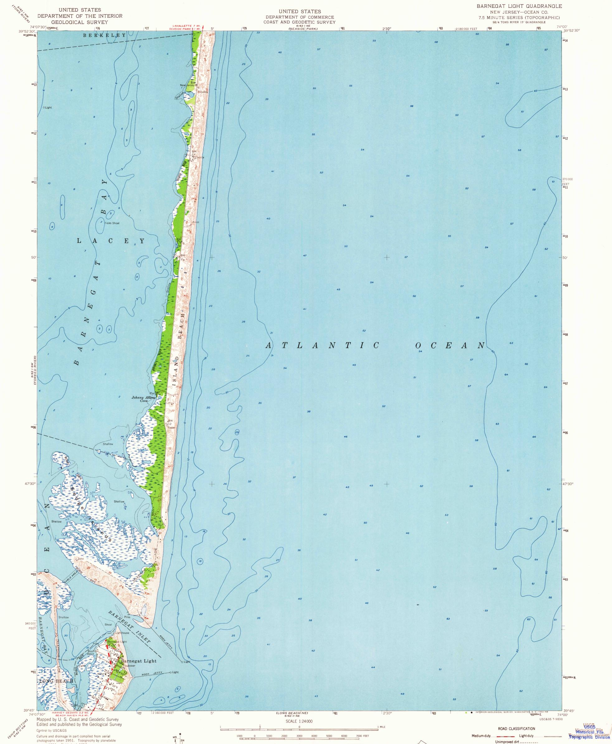
surveys 1951. Field check 1953 Hydrography compiled from USC&GS charts 825 (1953) and 1216 (1940) and surveys dated 1935, 1936, and 1937 Polyconic projection. 1927 North American datum 10,000-foot grid based on New Jersey coordinate system Unchecked elevations are shown in brown Island Beach borough boundary is low water line 1000-meter Universal Transverse Mercator grid ticks, zone 18, shown in blue
