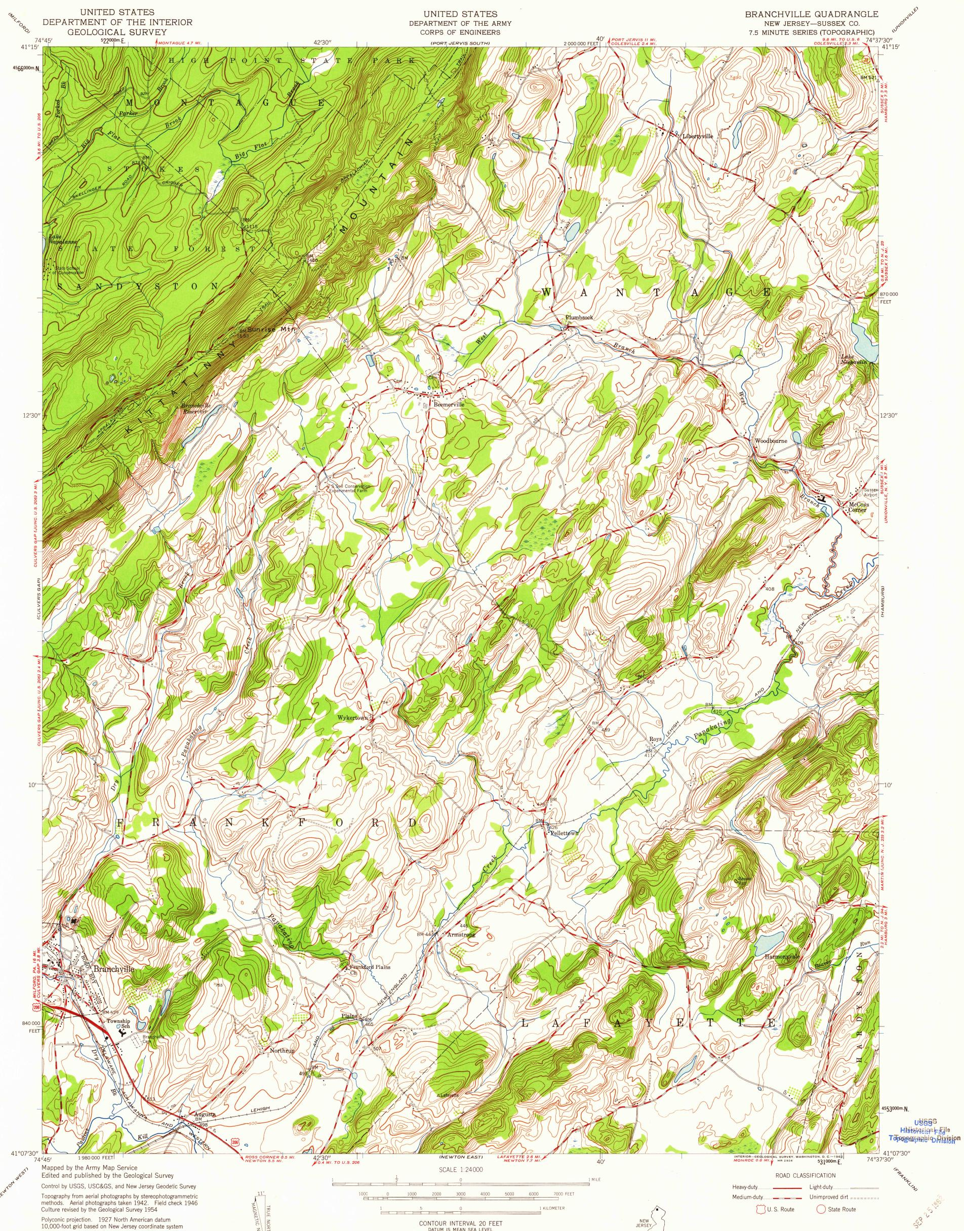
Polyconic projection. 1927 North American datum 10,000-foot grid based on New Jersey coordinate system Unchecked elevations are shown in brown 1000-meter Universal Transverse Mercator grid ticks, zone 18, shown in blue
