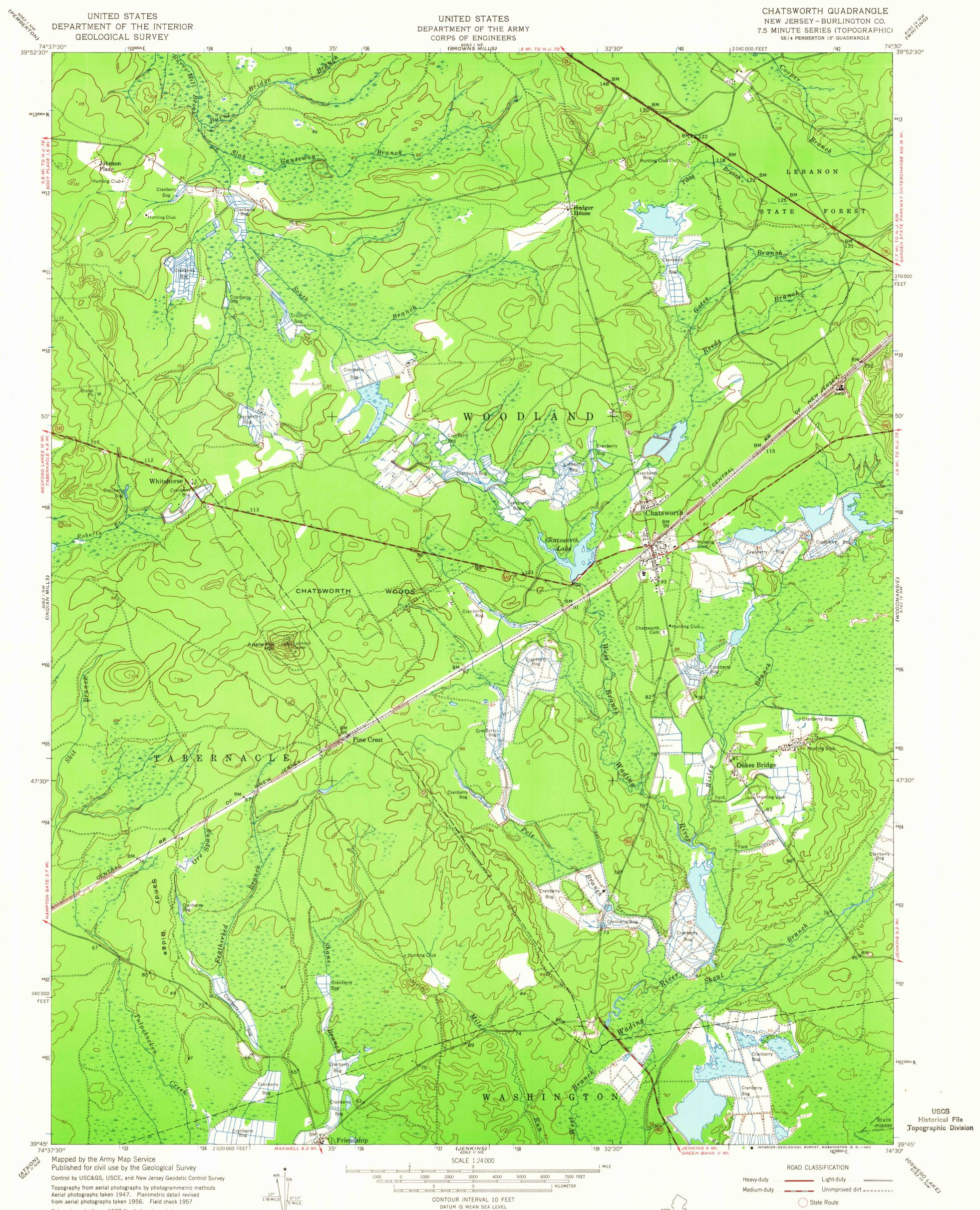
Polyconic projection. 1927 North American datum 10,000-foot grid based on New Jersey coordinate system 1000-meter Universal Transverse Mercator grid ticks, zone 18, shown in blue
