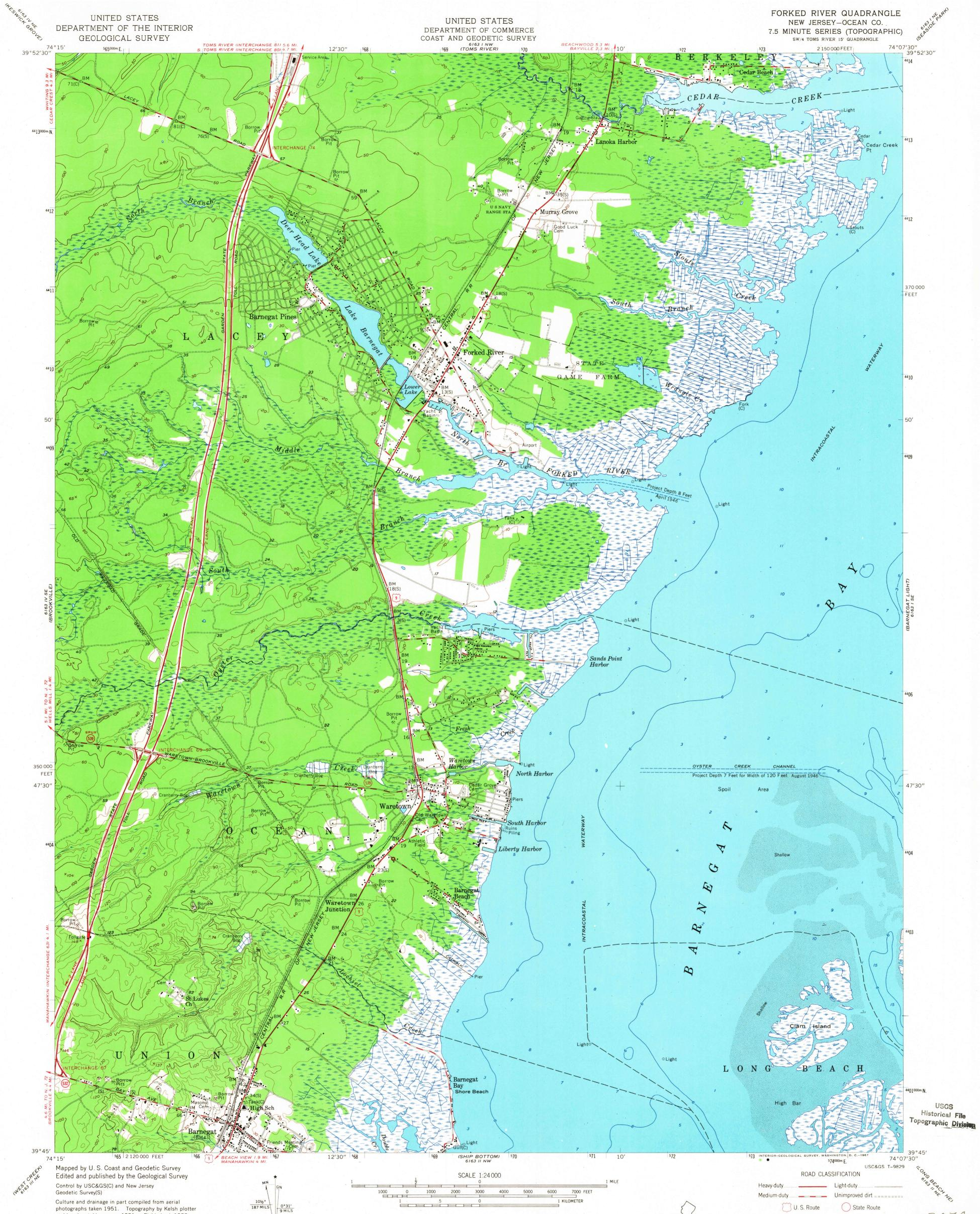
photographs taken 1951. Topography by Kelsh plotter and by planetable surveys 1951. Field check 1953 Hydrography compiled from USC&GS chart 825 (1954)
