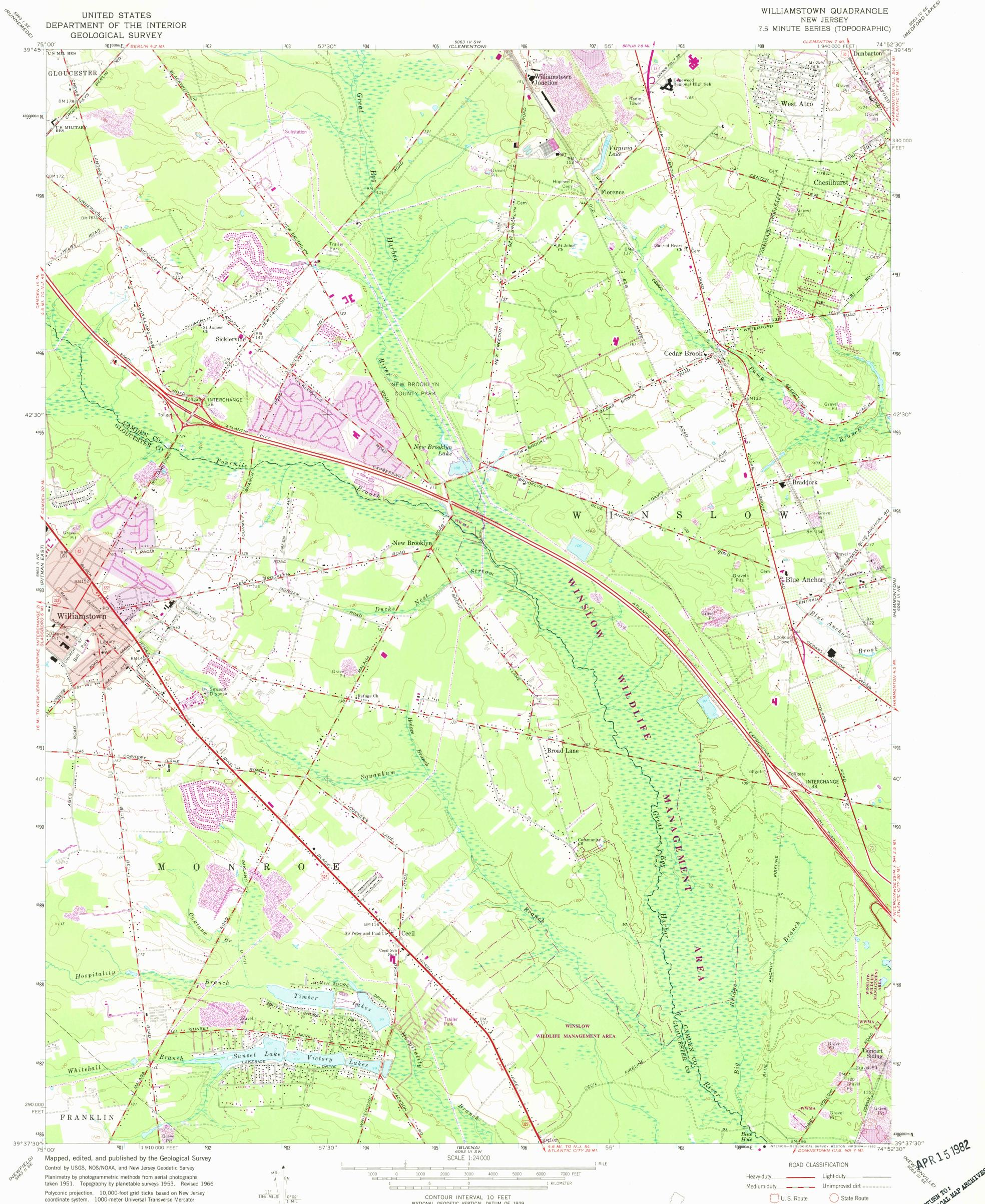
coordinate system. 1000-meter Universal Transverse Mercator grid ticks, zone 18, shown in blue. 1927 North American Datum. To place on the predicted North American Datum 1983 move the projection lines 6 meters south and 32 meters west as shown by dashed corner ticks
