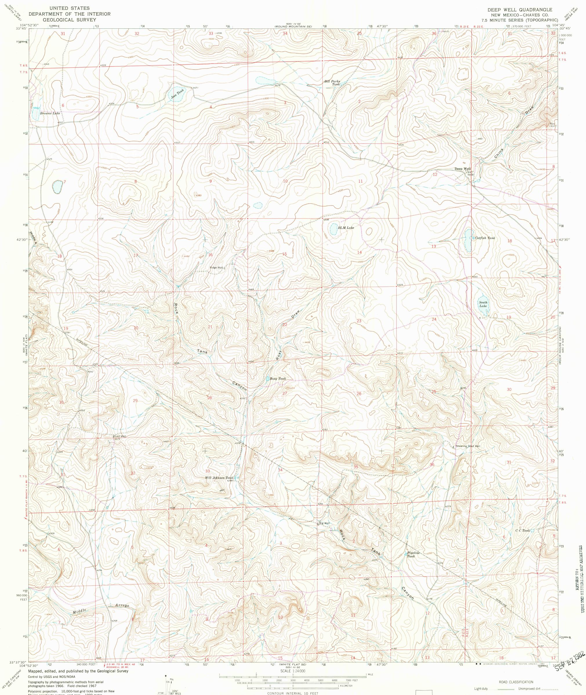
Mexico coordinate system, east zone. 1000-meter Universal Transverse Mercator grid ticks, zone 13, shown in blúe. 1927 North American Datum. To place on the predicted North American Datum 1983 move the projection lines 6 meters south and 48 meters east as shown by dashed corner ticks
