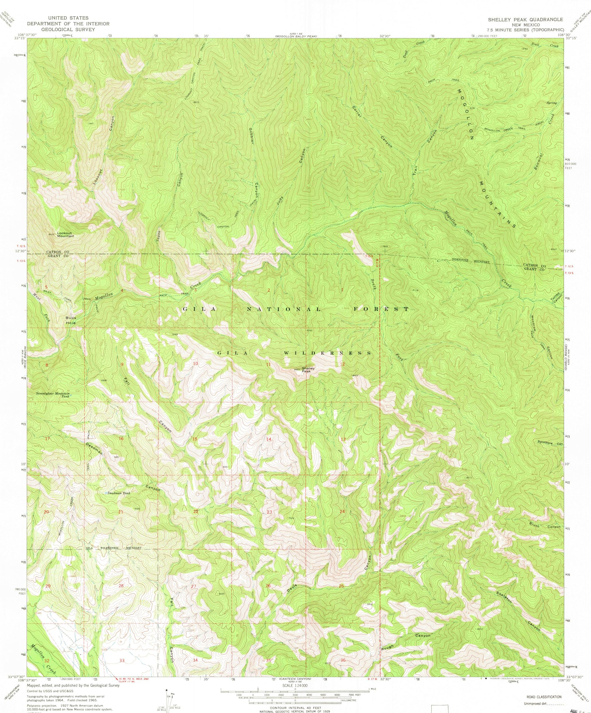
Polyconic projection. 1927 North American datum 10,000-foot grid based on New Mexico coordinate system, west zone 1000-metre Universal Transverse Mercator grid ticks, zone 12, shown in blue
