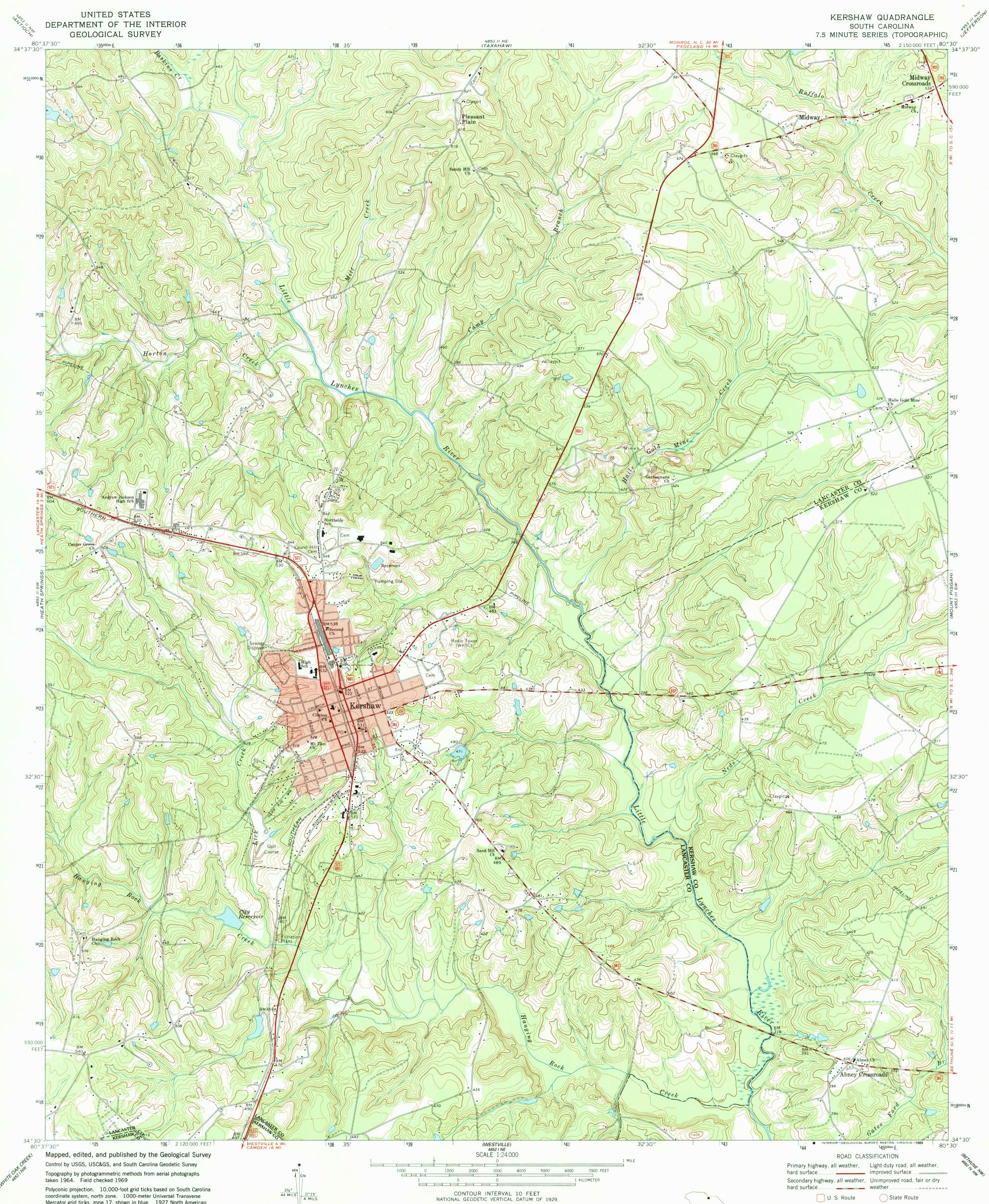
Mercator grid ticks, zone 17, shown in blue. 1927 North American Datum. To place on the predicted North American Datum 1983 move the projection lines 11 meters south and 18 meters west as shown by dashed corner ticks
