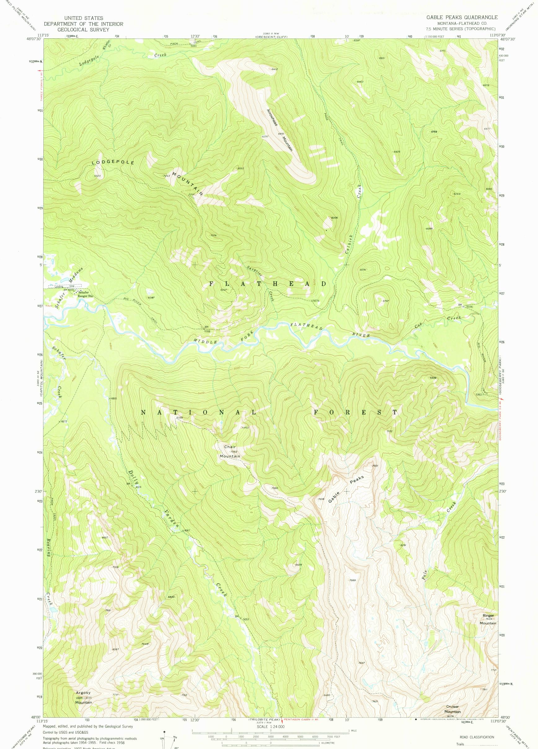
Polyconic projection. 1927 North American datum 10,000-foot grid based on Montana coordinate system, north zone 1000-metre Universal Transverse Mercator grid ticks, zone 12, shown in blue
