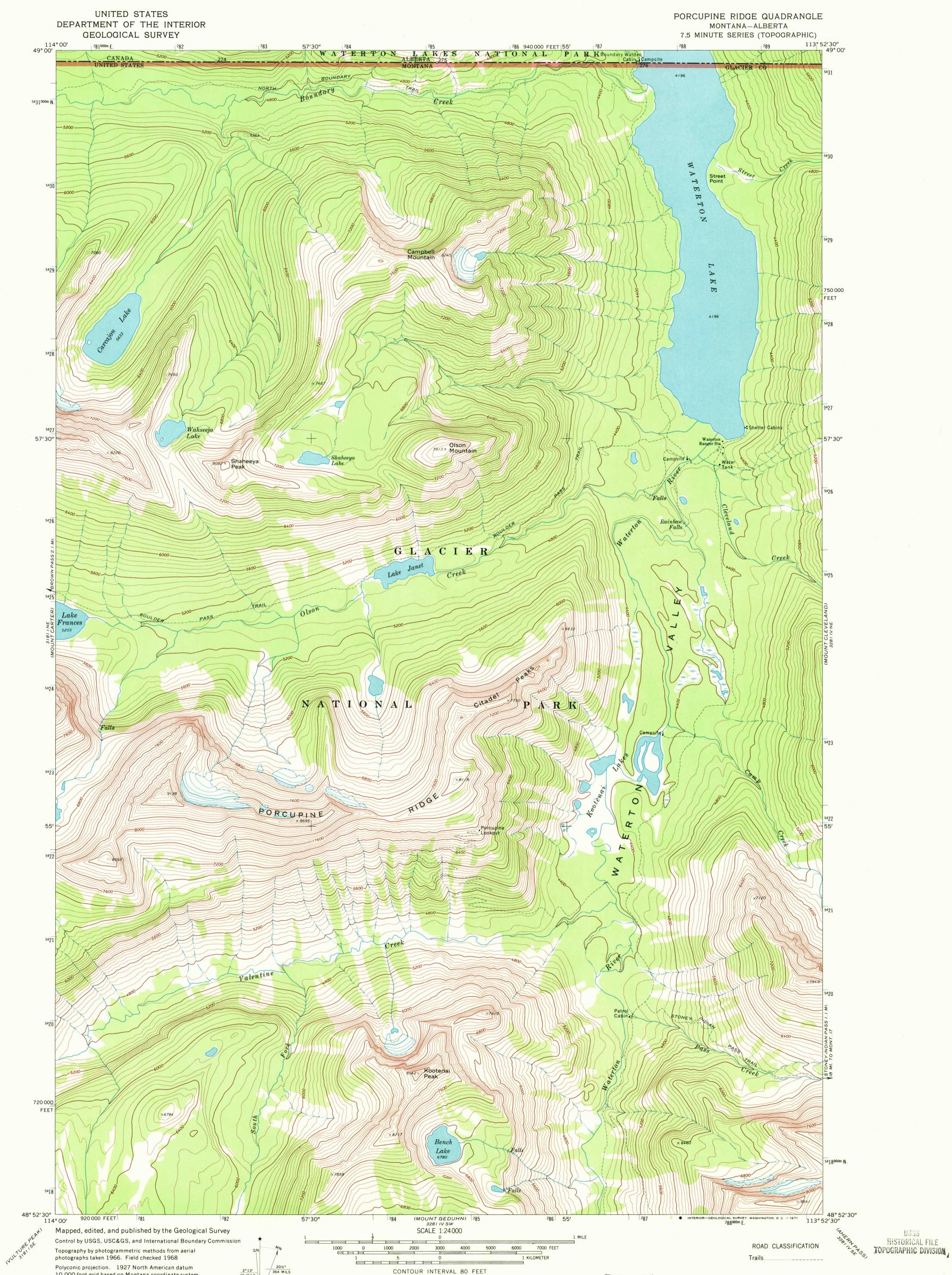
10,000-foot grid based on Montana coordinate system, north zone 1000-meter Universal Transverse Mercator grid ticks, zone 12, shown in blue Land lines have not been established in this area UTM GRID AND 1968 MAGNETIC NORTH DECLINATION AT CENTER OF SHEET
