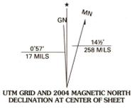
UTM GRID AND 2004 MAGNETIC NORTH DECLINATION AT CENTER OF SHEET
