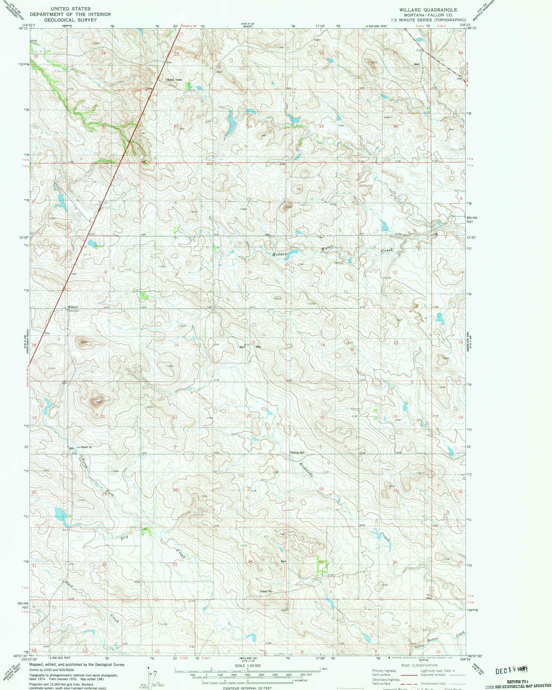
coordinate system, south zone (Lambert conformal conic) 1000-meter Universal Transverse Mercator grid, zone 13 1927 North American datum To place on the predicted North American Datum 1983 move the projection lines 4 meters north and 39 meters east as shown by dashed corner ticks
