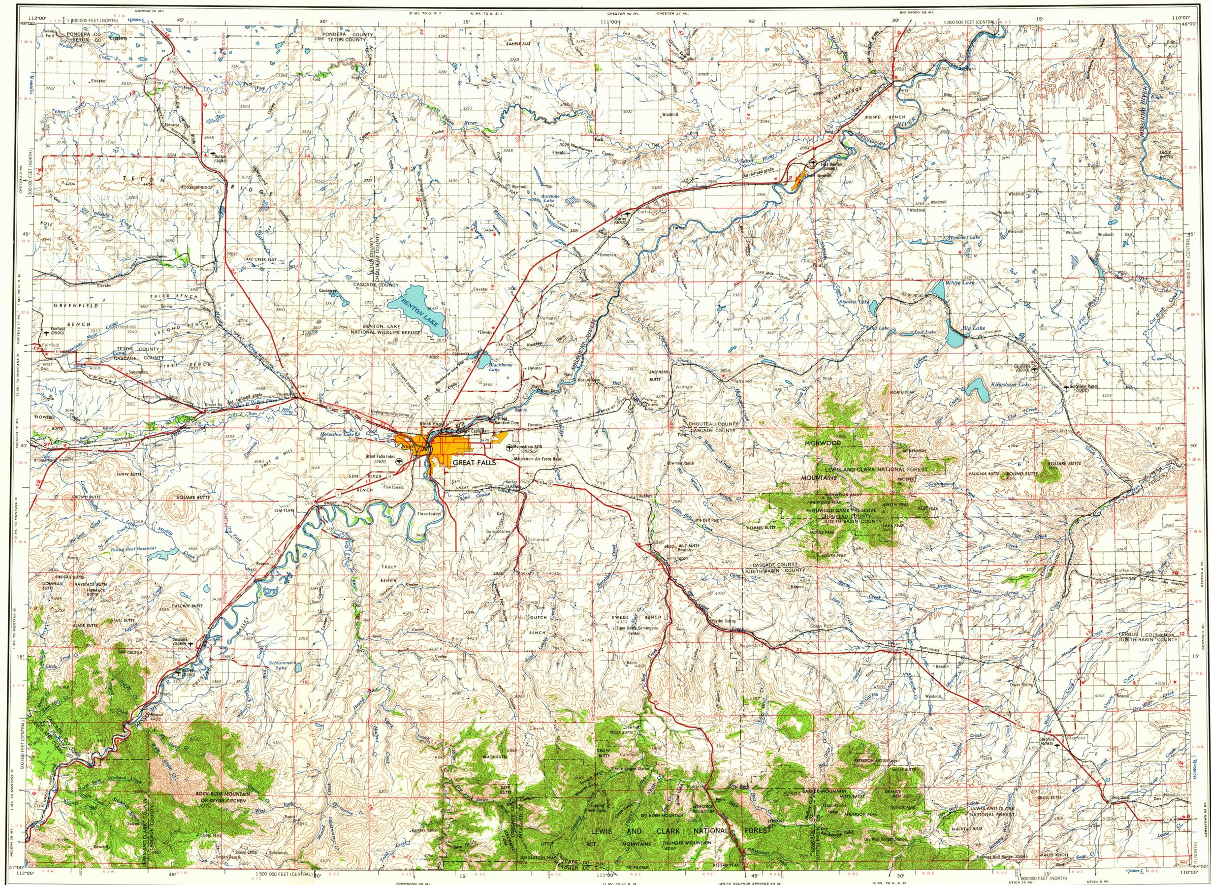
Prepared by the Army Map Service (AJAK1), Corps of Engineers, U.S. Army, Washington, D.C. Compiled in 1955 by photogrammetric methods. Horizontal and vertical control by USGS, USC&GS and USCE. Aerial photography 1953. Photography field annotated 1954. Limited revision by U.S. Geological Survey 1963.
