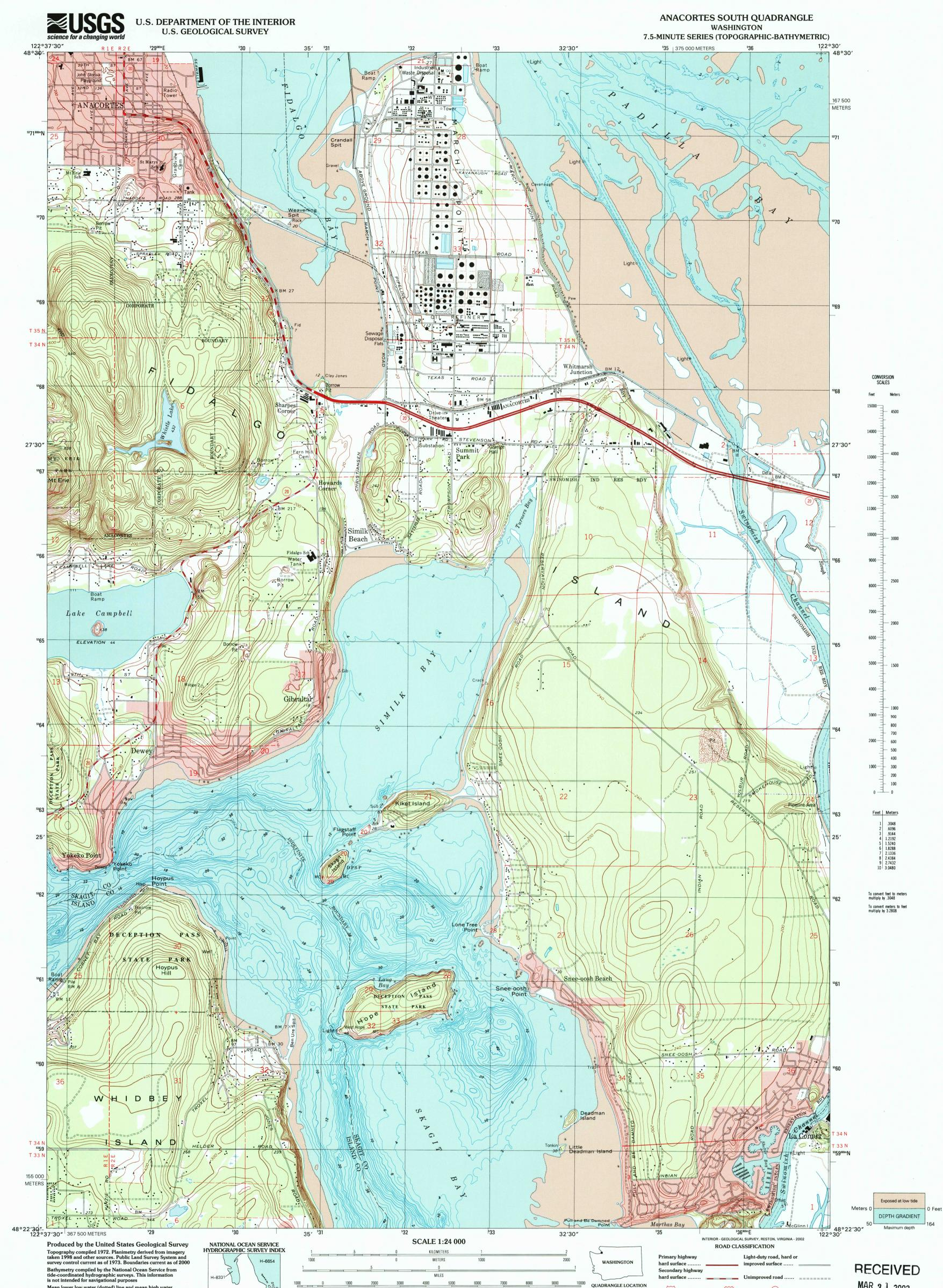
Mean lower low water (dotted) line and mean high water (solid) line compiled by NOS from tide-coordinated imagery
