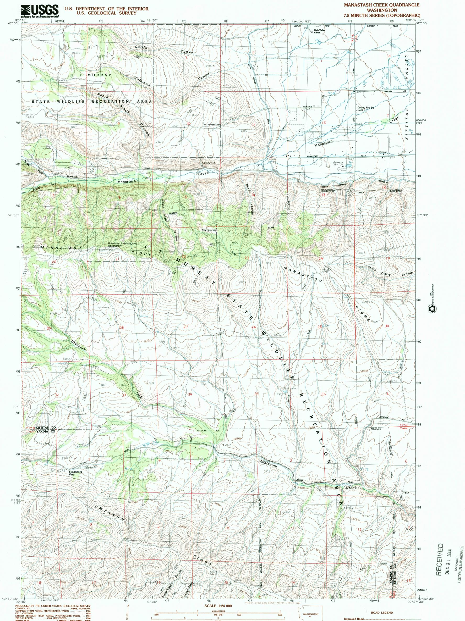
PROJECTION .. LAMBERT CONFORMAL CONIC To place on the predicted North American Datum of 1983, move the projection lines as shown by dashed corner ticks (20 meters north/89 meters east) There may be private inholdings within the boundaries of any Federal and State Reservations shown on this map
