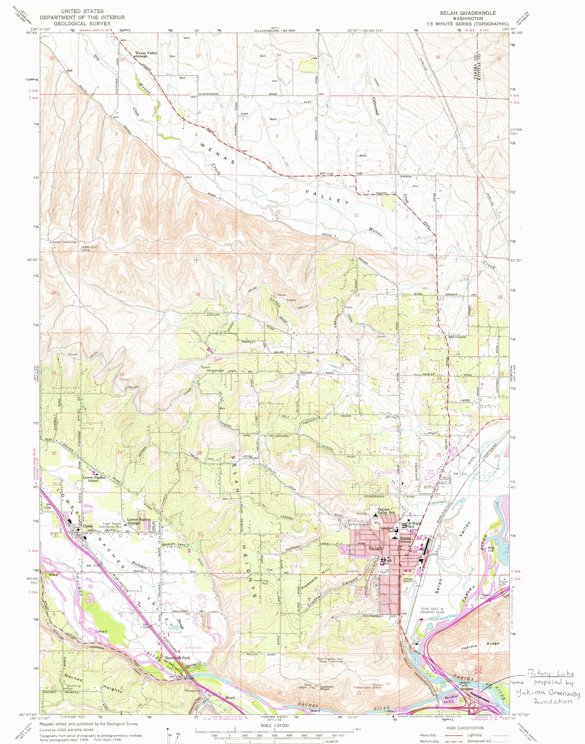
Polyconic projection. 1927 North American datum 1°46' 31 MILS 10,000-foot grid based on Washington coordinate system, south zone 1000-metre Universal Transverse Mercator grid ticks, zone 10, shown in blue Red tint indicates area in which only UTM GRID AND 1974 MAGNETIC NORTH DECLINATION AT CENTER OF SHEET landmark buildings are shown Revisions shown in purple compiled from aerial photographs taken 1974. This information not field checked Purple tint indicates extension of urban areas
