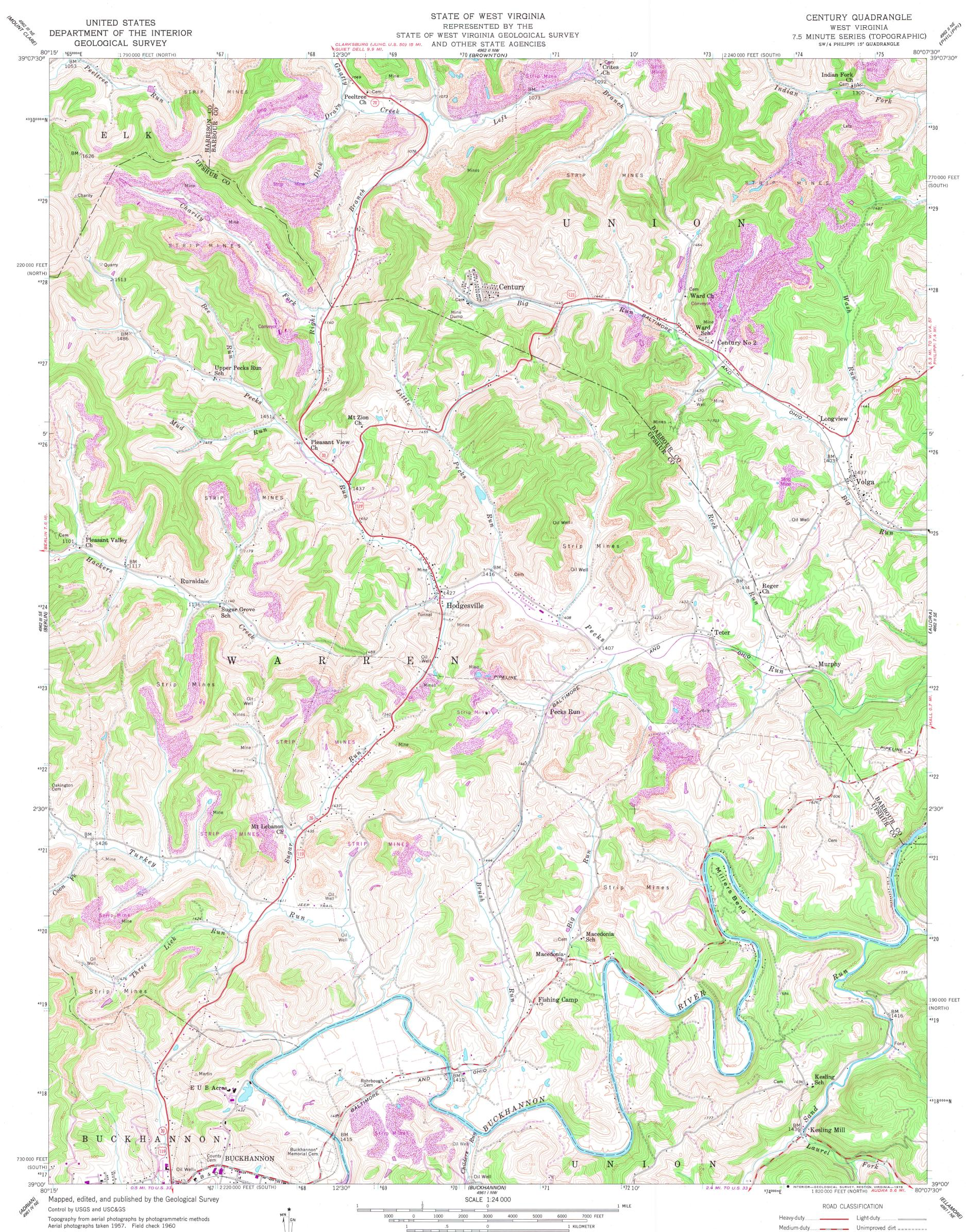
Aerial photographs taken 1957. Field check 1960 Polyconic projection. 1927 North American datum 10,000-foot grid based on West Virginia coordinate system, south and north zones 1000-meter Universal Transverse Mercator grid ticks, zone 17, shown in blue Fine red dashed lines indicate selected fence and field lines where generally visible on aerial photographs. This information is unchecked
