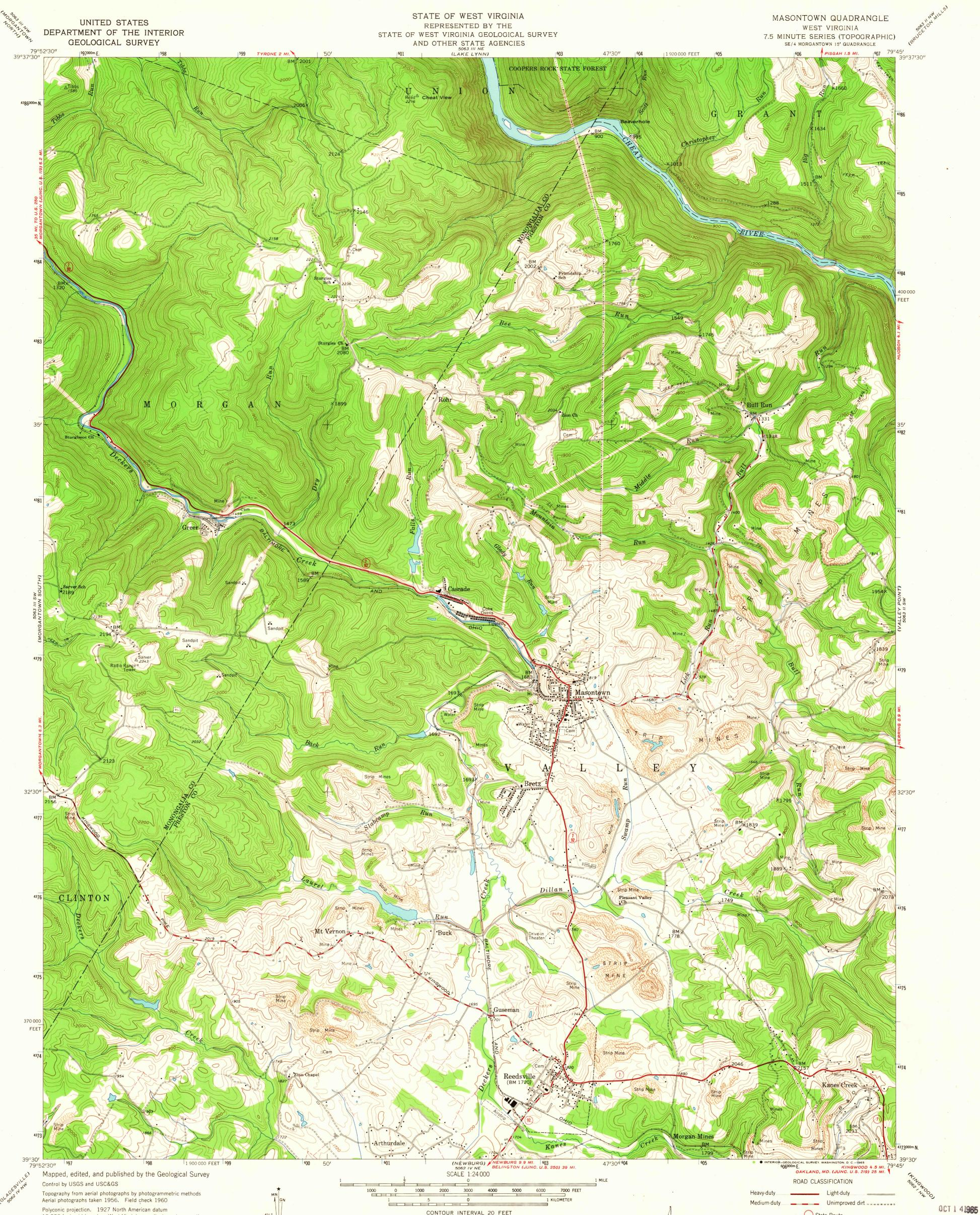
Polyconic projection. 1927 North American datum 10,000-foot grid based on West Virginia coordinate system, north zone 1000-meter Universal Transverse Mercator grid ticks, zone 17, shown in blue
