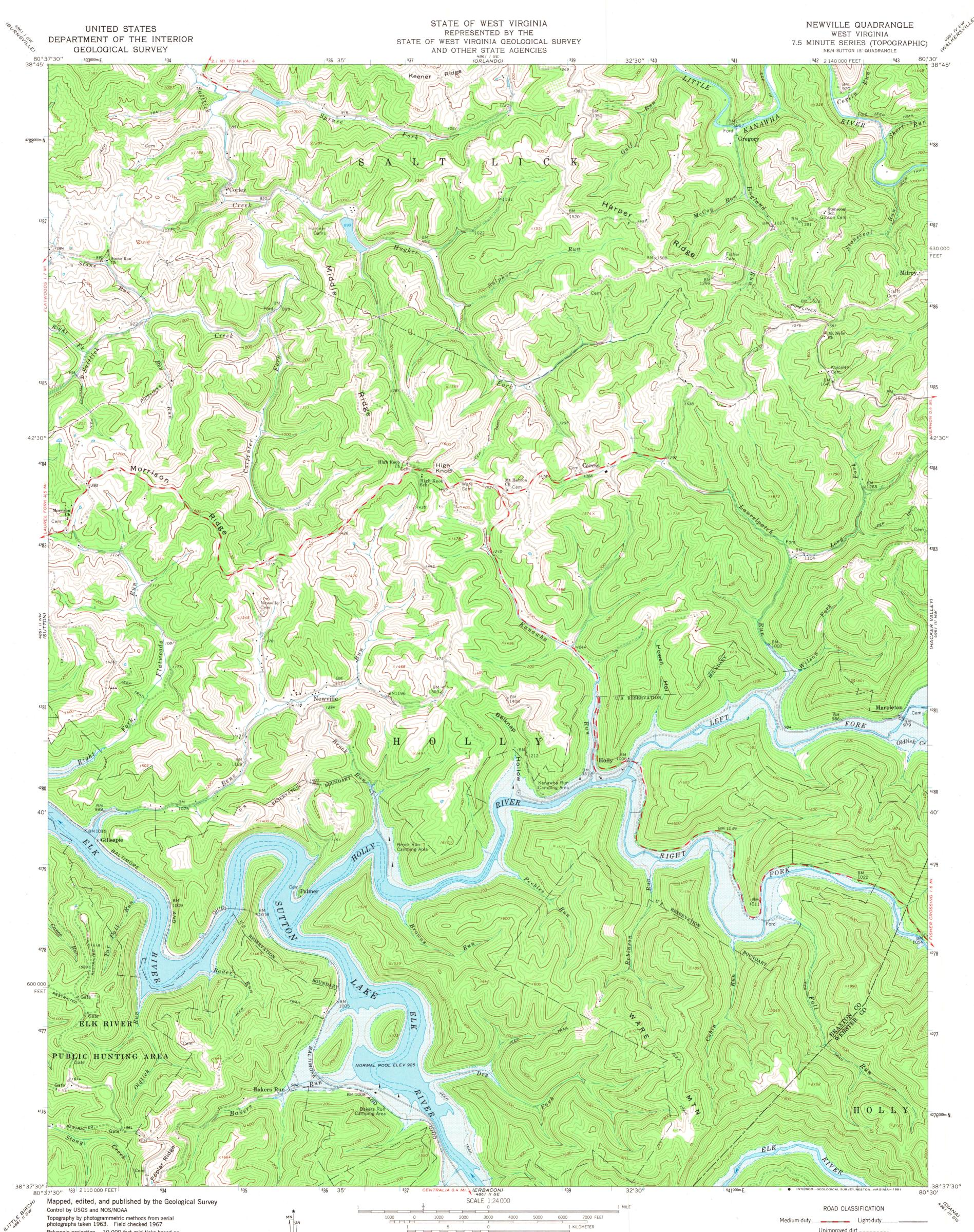
Polyconic projection. 10,000-foot grid ticks based on West Virginia coordinate system, south zone 1000-meter Universal Transverse Mercator grid ticks, zone 17, shown in blue. 1927 North American Datum To place on the predicted North American Datum 1983 move the projection lines 7 meters south and 17 meters west as shown by dashed corner ticks
