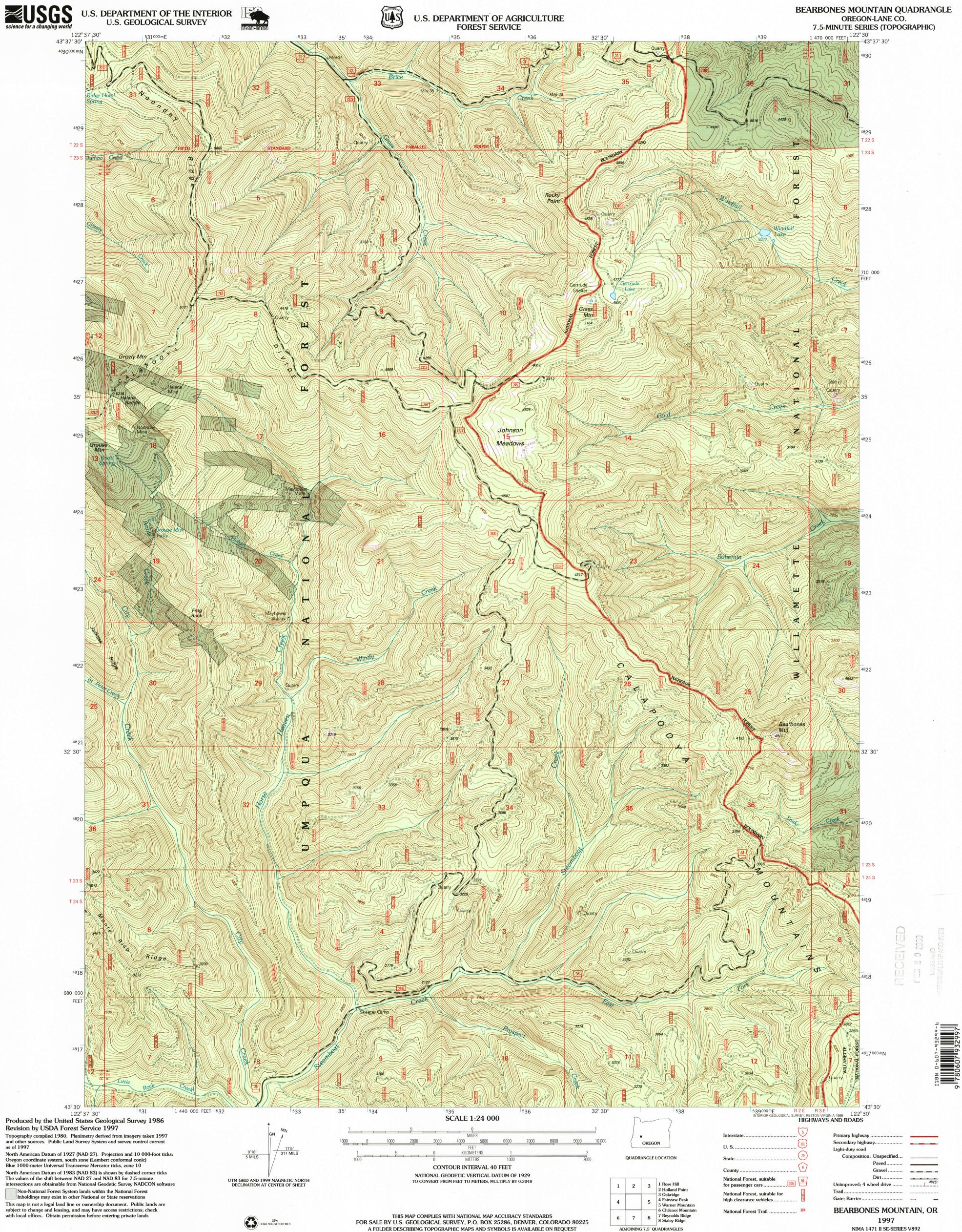
Blue 1000-meter Universal Transverse Mercator ticks, zone 10 North American Datum of 1983 (NAD 83) is shown by dashed corner ticks The values of the shift between NAD 27 and NAD 83 for 7.5-minute intersections are obtainable from National Geodetic Survey NADCON software
