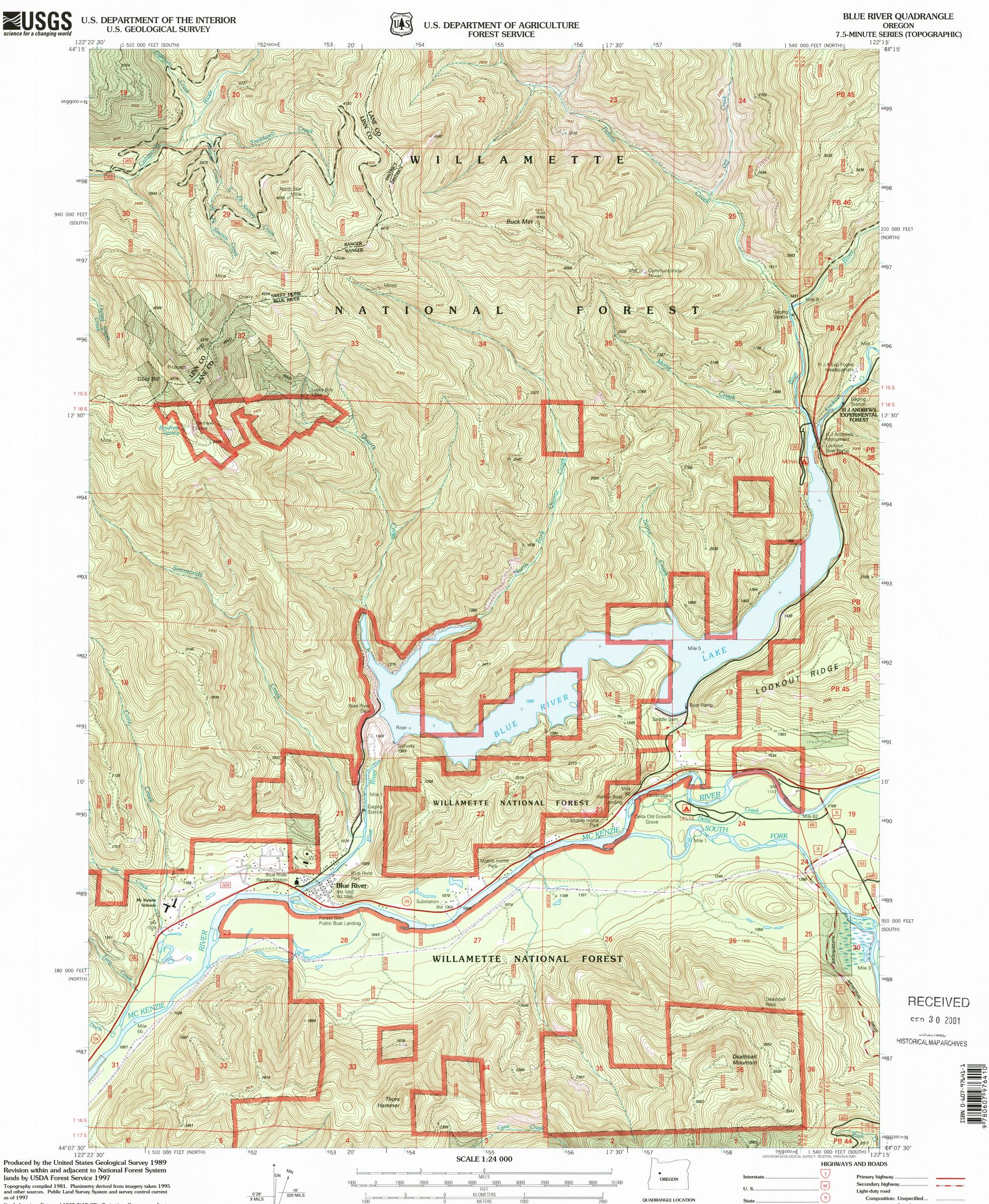
North American Datum of 1927 (NAD 27). Projection: Oregon coordinate system, north zone (Lambert conformal conic). 10 000-foot ticks: Oregon coordinate system, north and south zones. Blue 1000-meter Universal Transverse Mercator ticks, zone 10
