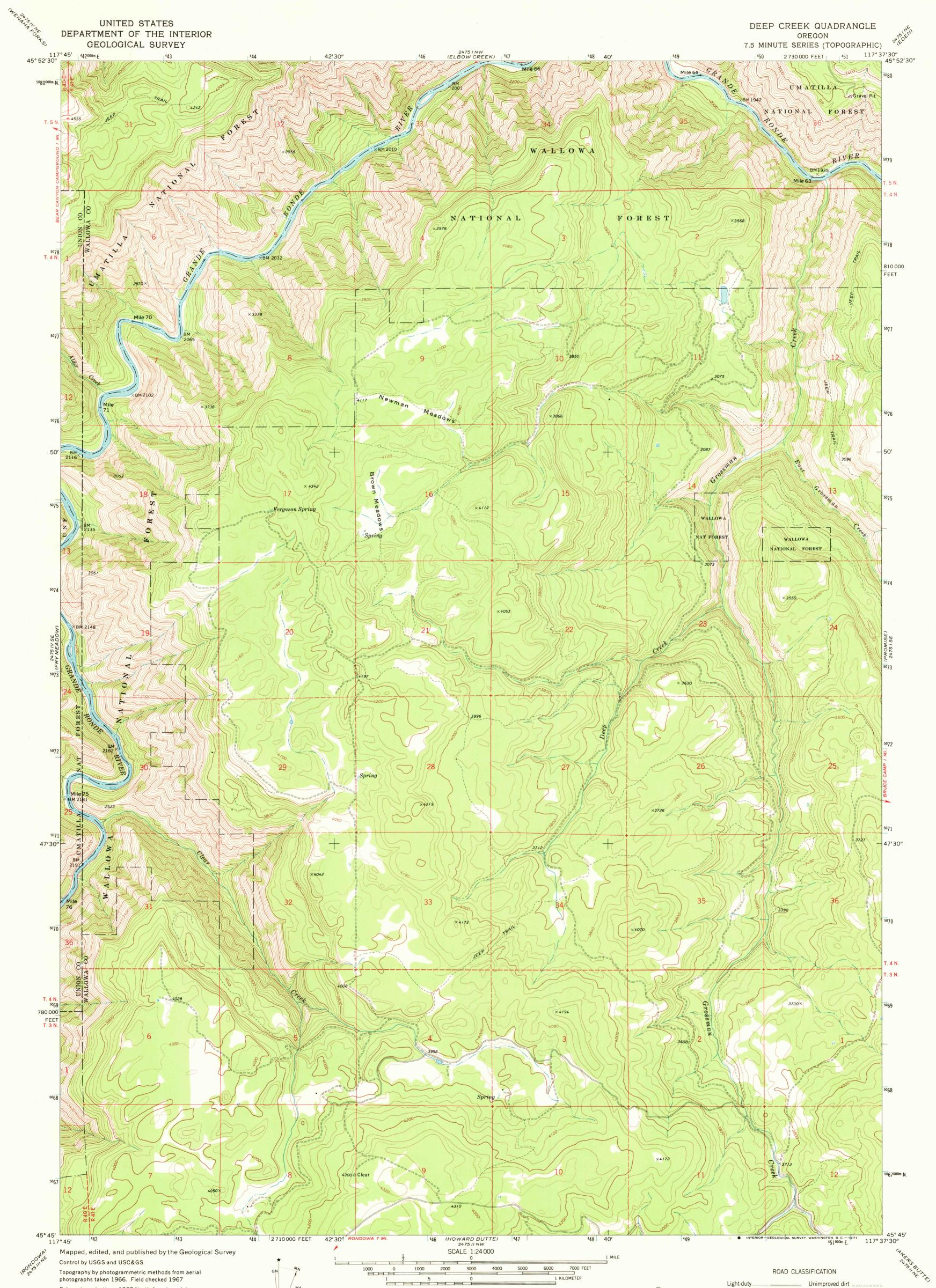
Polyconic projection. 1927 North American datum 10,000-foot grid based on Oregon coordinate system, north zone 1000-meter Universal Transverse Mercator grid ticks, zone 11, shown in blue
