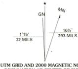
UTM GRID AND 2000 MAGNETIC NORTH DECLINATION AT CENTER OF SHEET
