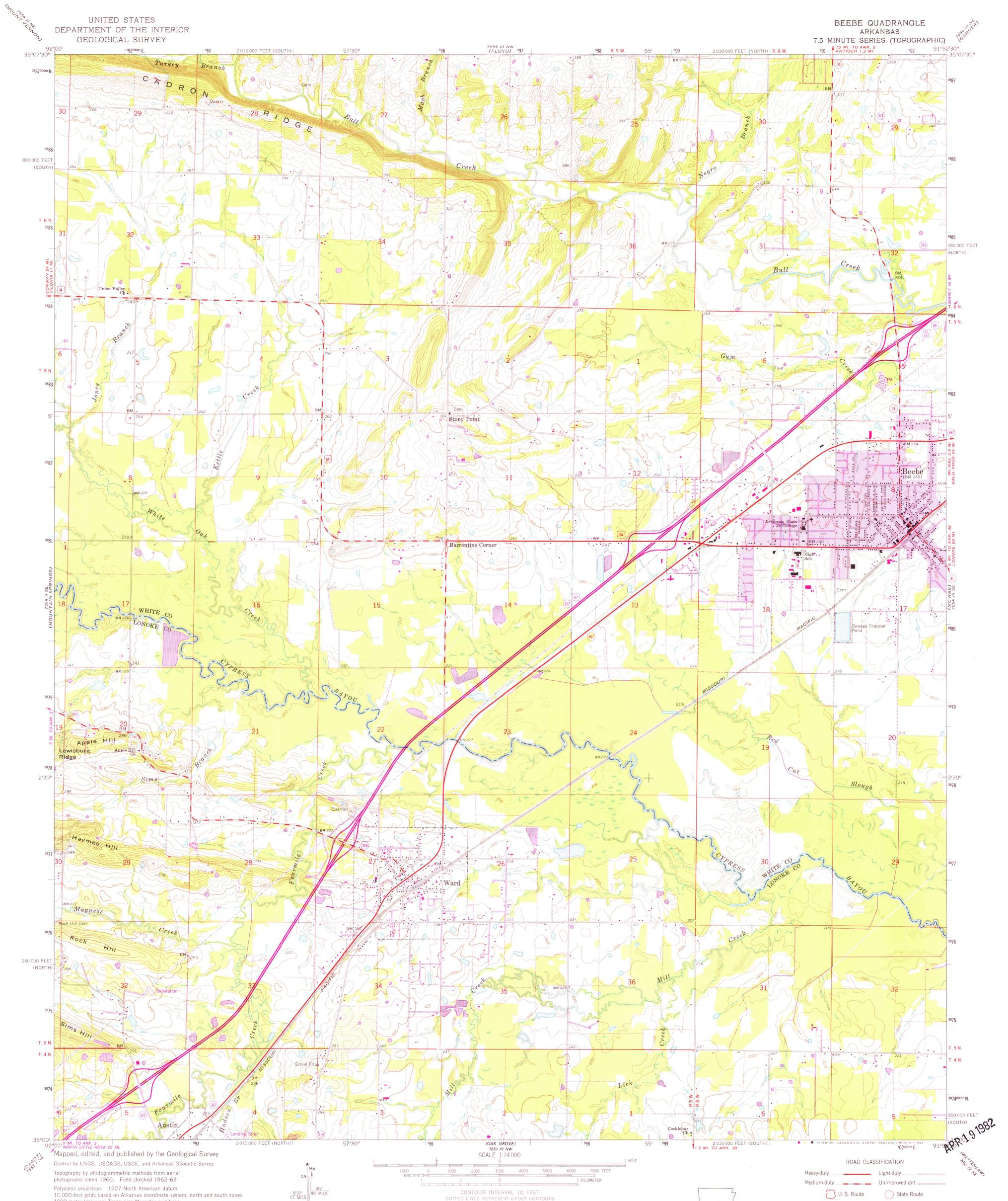
10,000-foot grids based on Arkansas coordinate system, north and south zones 1000-meter Universal Transverse Mercator grid ticks, zone 15, shown in blue
