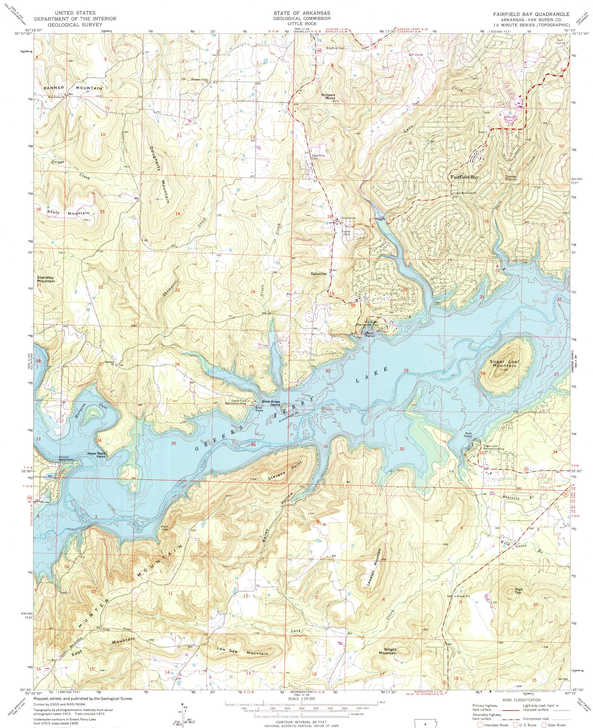
Projection and 10,000-foot grid ticks: Arkansas coordinate system, north zone (Lambert conformal conic) 1000-metre Universal Transverse Mercator grid ticks, zone 15, shown in blue. 1927 North American datum
