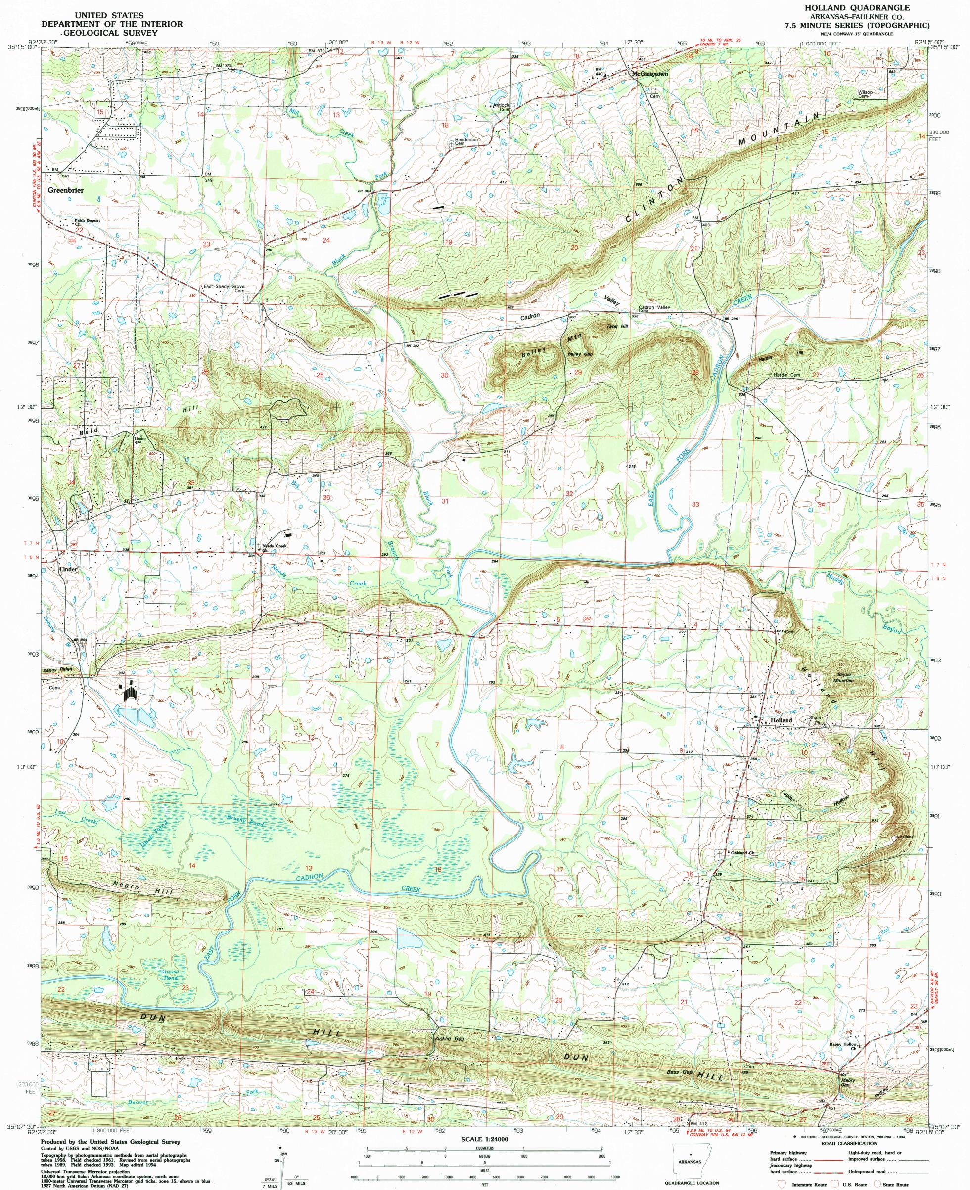
North American Datum of 1983 (NAD 83) is shown by dashed corner ticks The values of the shift between NAD 27 and NAD 83 for 7.5-minute intersections are given in USGS Bulletin 1875
