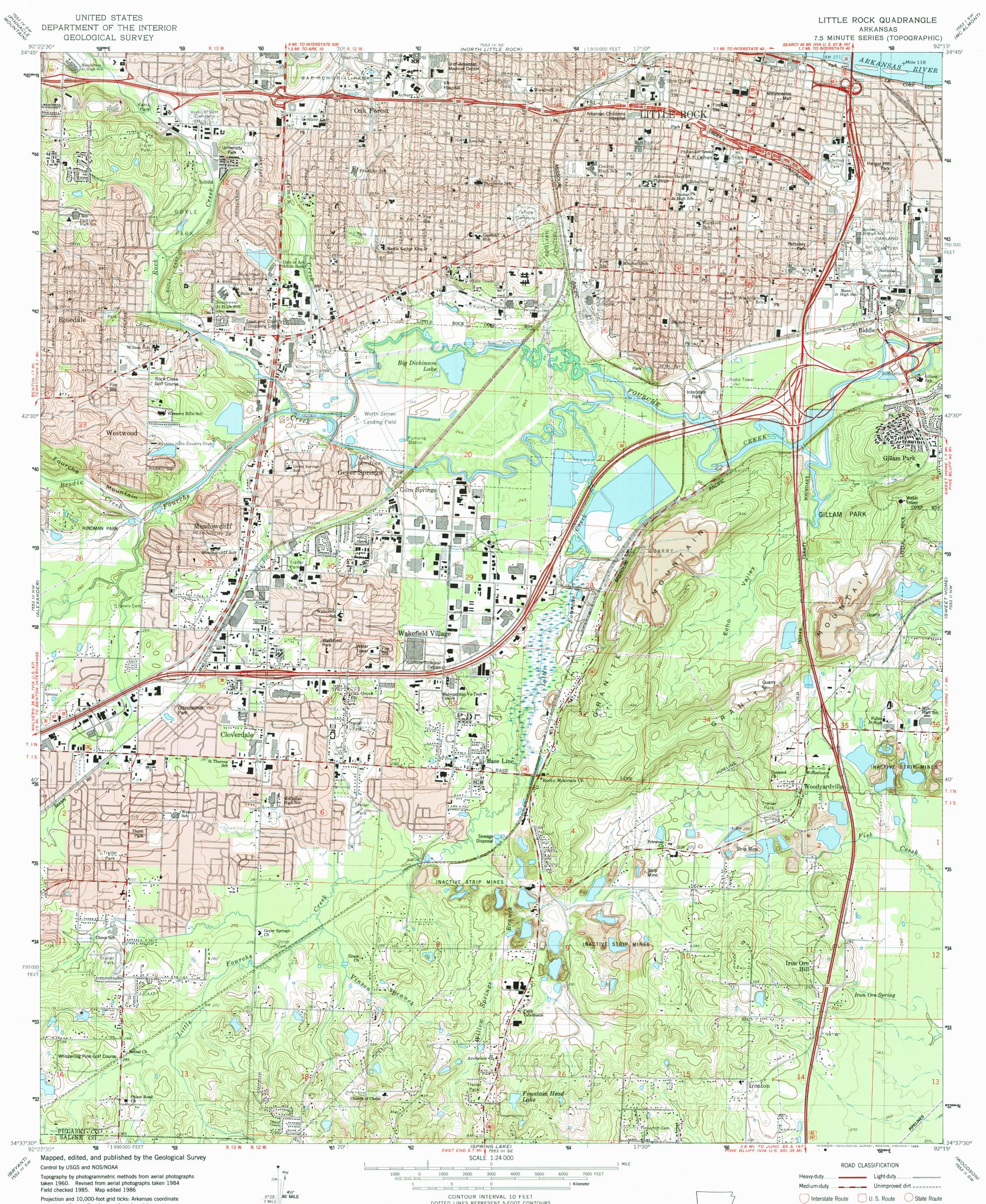
Projection and 10,000-foot grid ticks: Arkansas coordinate system, south zone (Lambert conformal conic) 1000-meter Universal Transverse Mercator grid, zone 15 1927 North American Datum To place on the predicted North American Datum 1983, move the projection lines 7 meters south and 14 meters east as shown by dashed corner ticks Red tint indicates areas in which only landmark buildings are shown
