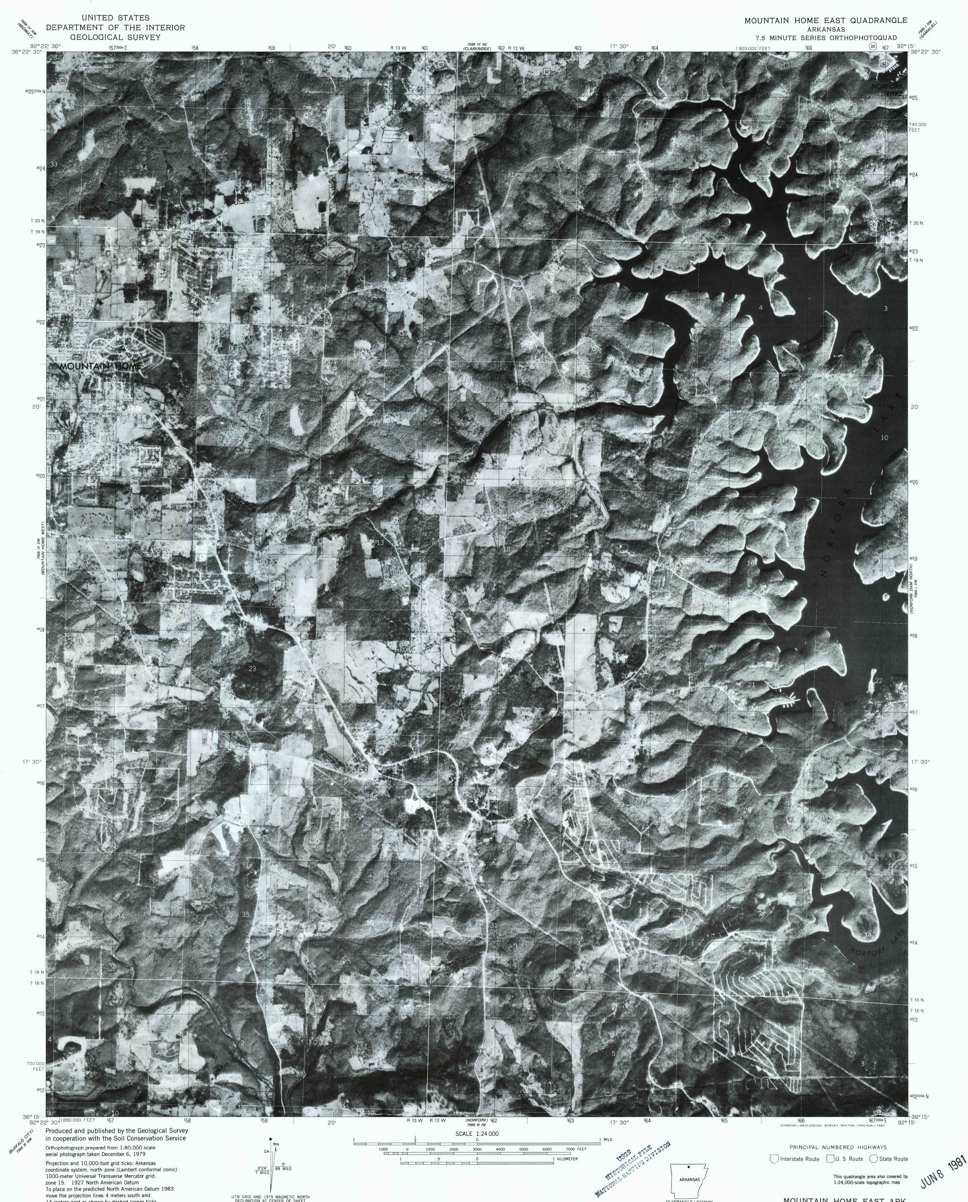
coordinate system, north zone (Lambert conformal conic) 1000-meter Universal Transverse Mercator grid, zone 15. 1927 North American Datum To place on the predicted North American Datum 1983 move the projection lines 4 meters south and 14 meters east as shown by dashed corner ticks
