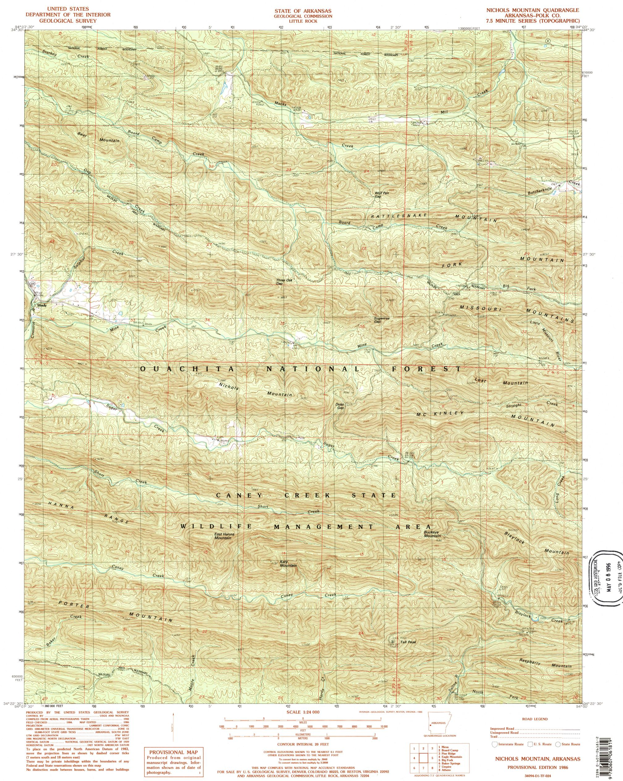
1986 MAGNETIC NORTH DECLINATION .... . 5°30' EAST VERTICAL DATUM ...... NATIONAL GEODETIC VERTICAL DATUM OF 1929 HORIZONTAL DATUM ...... 1927 NORTH AMERICAN DATUM To place on the predicted North American Datum of 1983, move the projection lines as shown by dashed corner ticks (7 meters south and 18 meters east) There may be private inholdings within the boundaries of any Federal and State reservations shown on this map No distinction made between houses, barns, and other buildings
