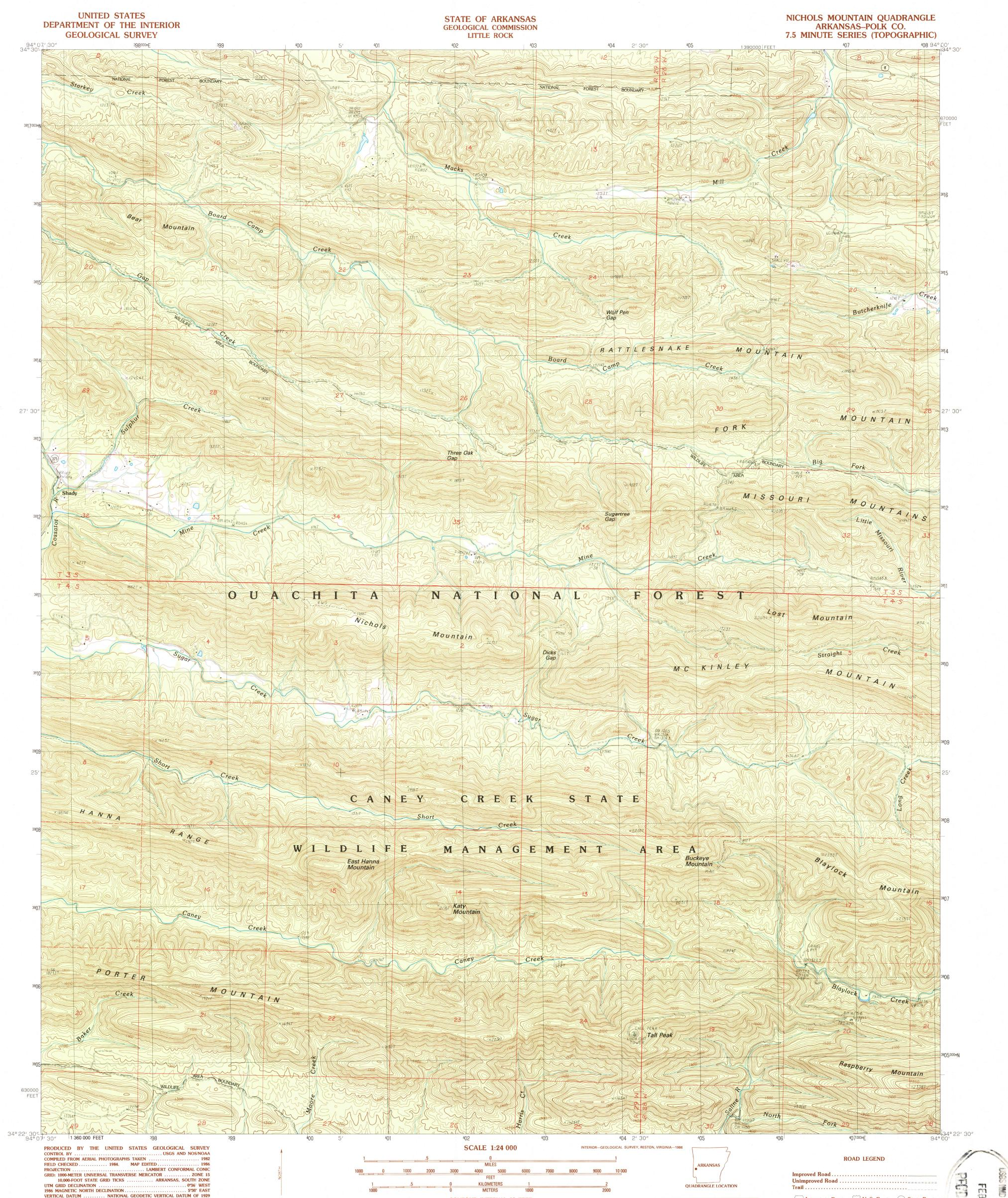
1986 MAGNETIC NORTH DECLINATION ..... .. 5°30' EAST VERTICAL DATUM ..... NATIONAL GEODETIC VERTICAL DATUM OF 1929 ..... 1927 NORTH AMERICAN DATUM HORIZONTAL DATUM ... To place on the predicted North American Datum of 1983, move the projection lines as shown by dashed corner ticks (7 meters south and 18 meters east) There may be private inholdings within the boundaries of any Federal and State reservations shown on this map No distinction made between houses, barns, and other buildings
