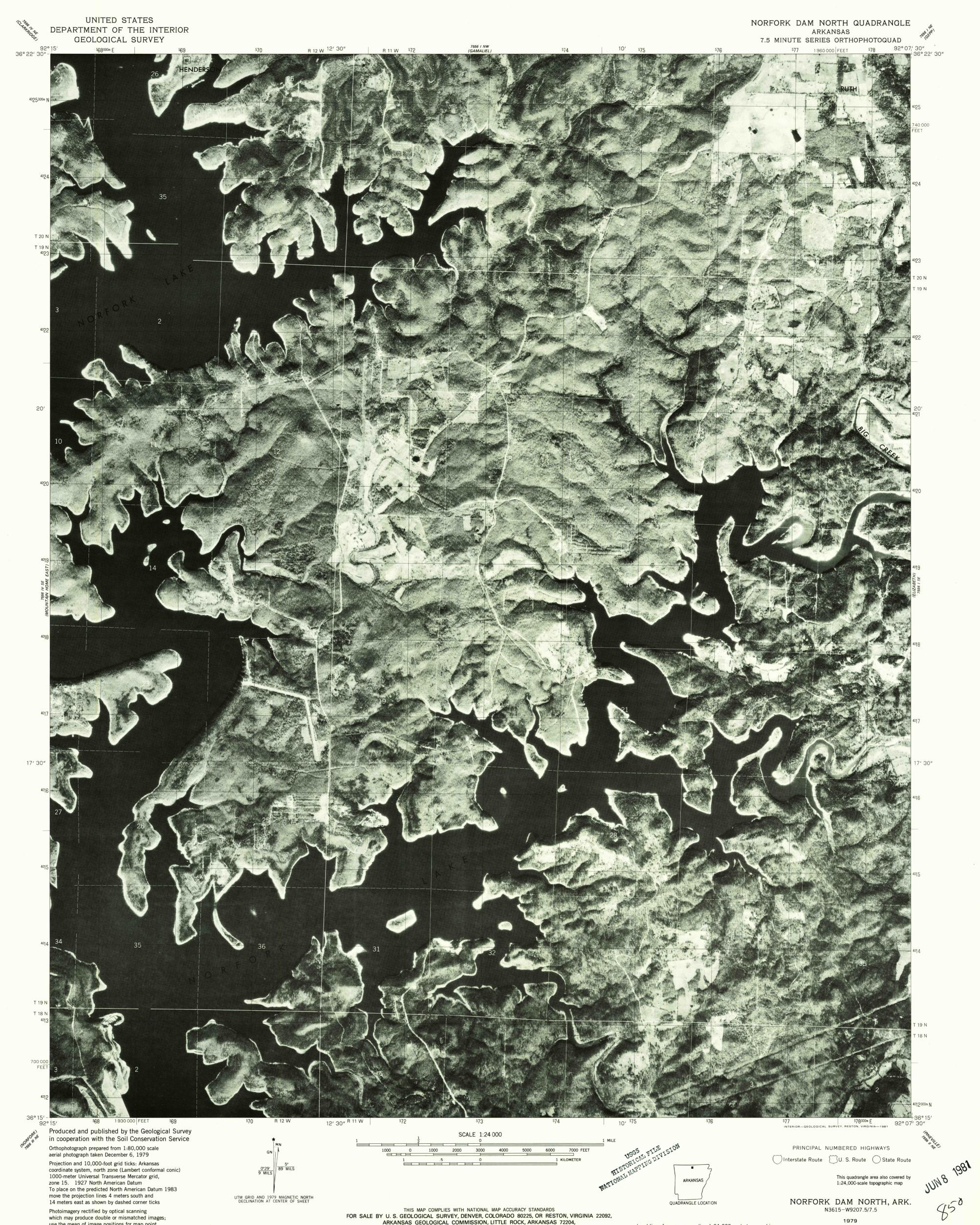
1000-meter Universal Transverse Mercator grid, zone 15. 1927 North American Datum To place on the predicted North American Datum 1983 move the projection lines 4 meters south and 14 meters east as shown by dashed corner ticks Photoimagery rectified by optical scanning
