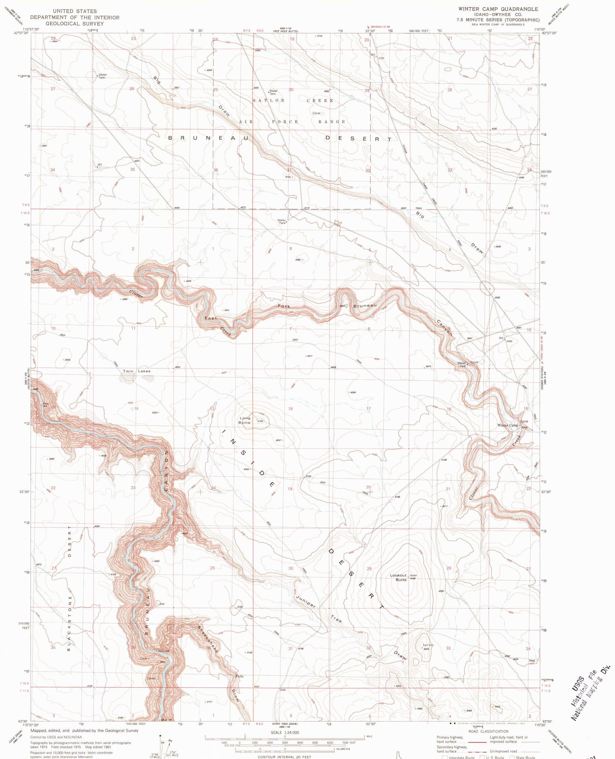
Projection and 10,000-foot grid ticks: Idaho coordinate system, west zone (transverse Mercator) 1000-meter Universal Transverse Mercator grid, zone 11 1927 North American Datum To place on the predicted North American Datum 1983 move the projection lines 14 meters north and 75 meters east as shown by dashed corner ticks
