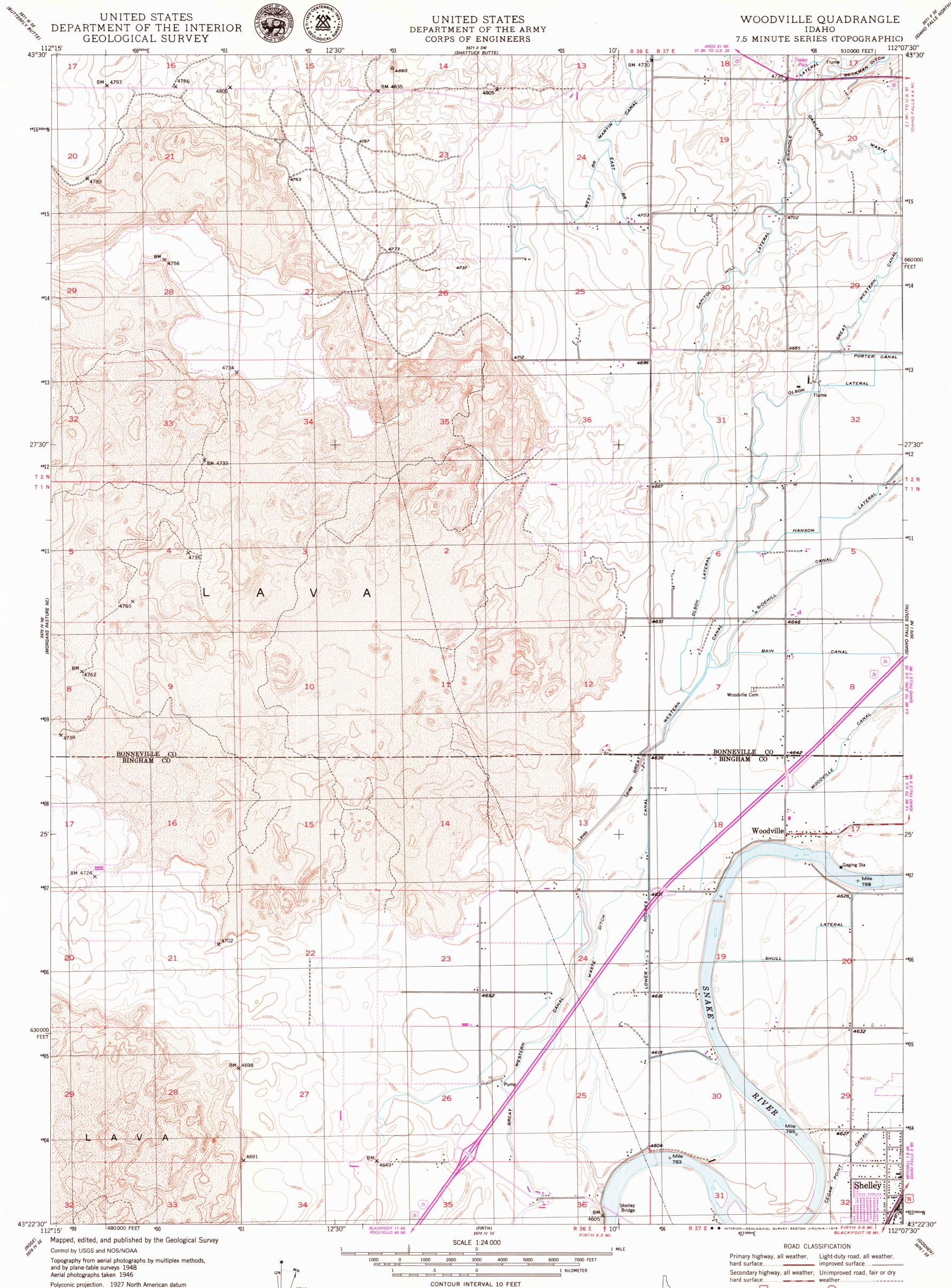
10,000-foot grid based on Idaho coordinate system, east zone 1000-meter Universal Transverse Mercator grid, zone 12, 1927 North American datum To place on the predicted North American Datum 1983, move the projection lines 12 meters north and 66 meters east as shown by dashed corner ticks 16½°
