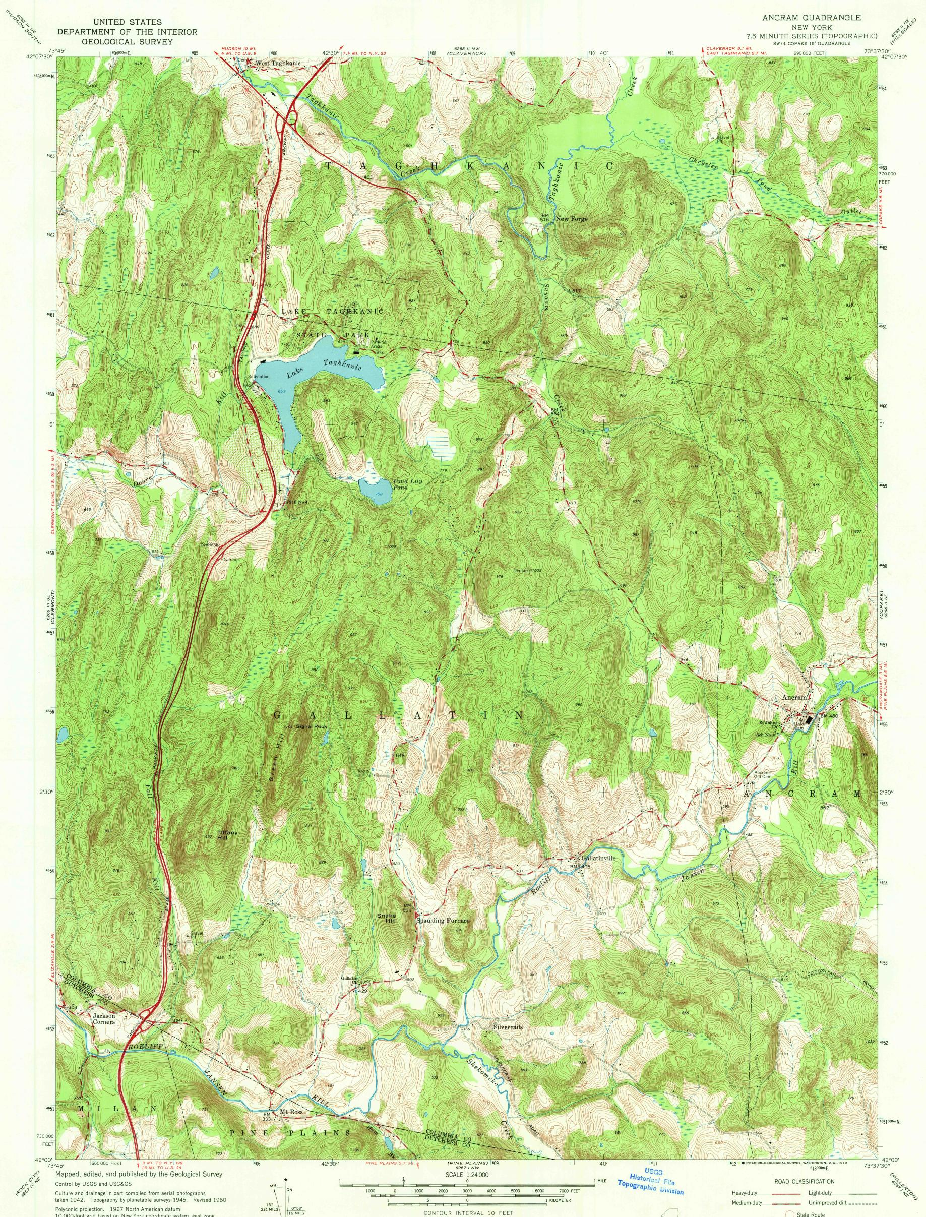
Polyconic projection. 1927 North American datum 10,000-foot grid based on New York coordinate system, east zone 1000-meter Universal Transverse Mercator grid ticks, zone 18, shown in blue
