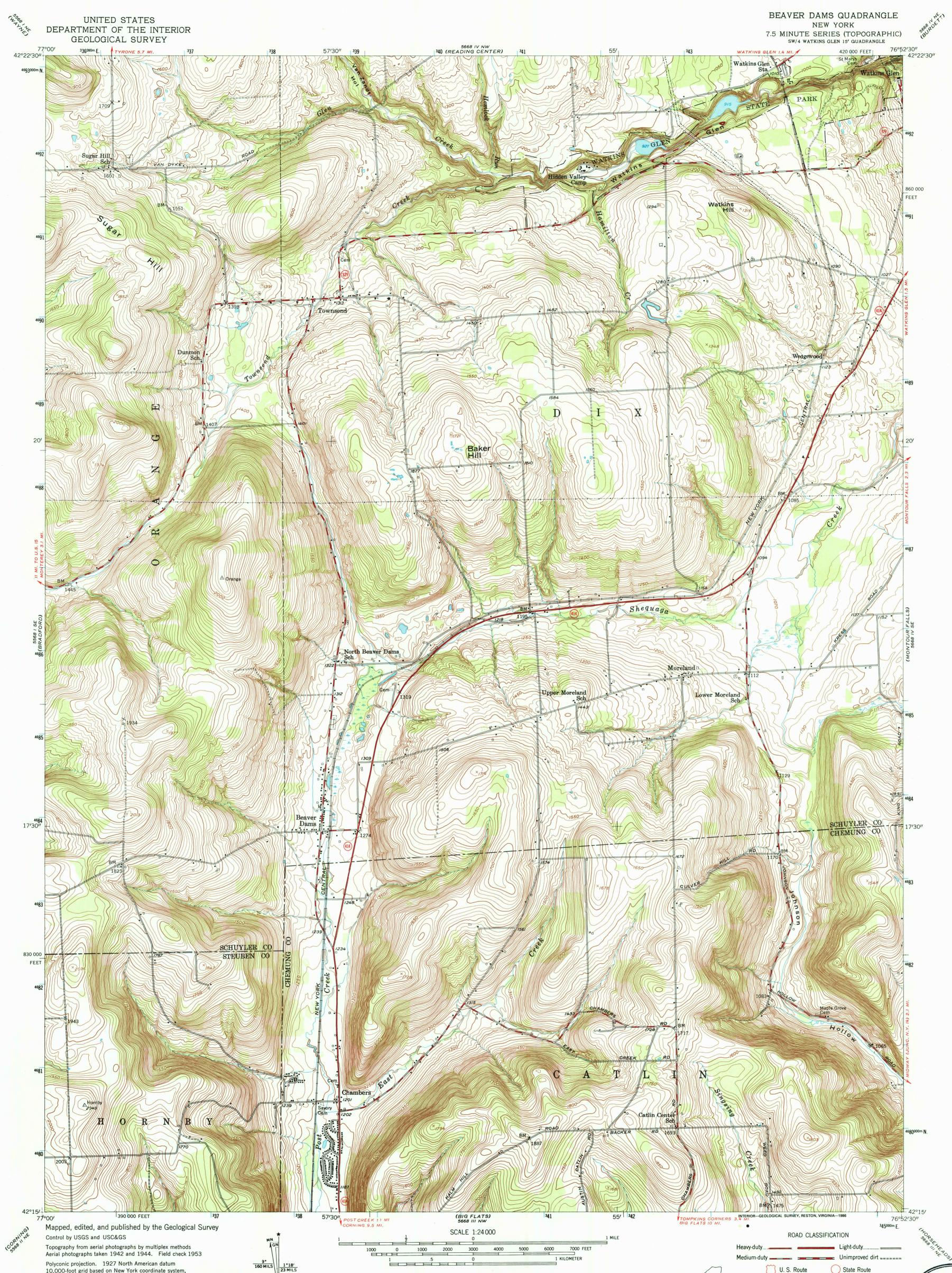
Polyconic projection. 1927 North American datum 10,000-foot grid based on New York coordinate system, central zone 1000-meter Universal Transverse Mercator grid ticks, zone 18, shown in blue To place on the predicted North American Datum 1983, move the projection lines 3 meters south and
