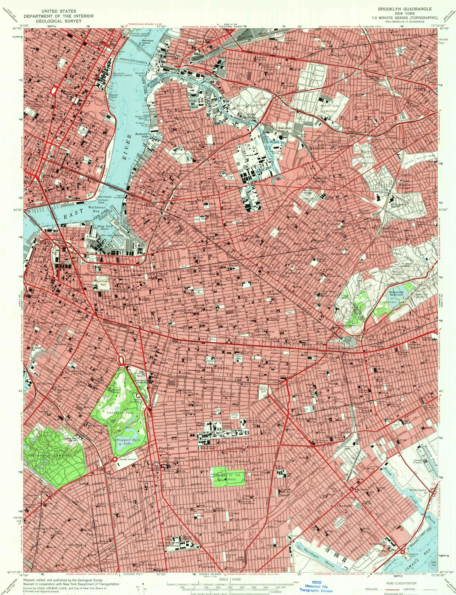
Planimetry by photogrammetric methods from aerial photographs taken 1954, and from USC&GS Charts T-5094, T-5335, T-5454 T-5459, T-5460, and T-8449 Topography by planetable surveys 1955–1956. Revised from aerial photographs taken 1966. Field checked 1967
